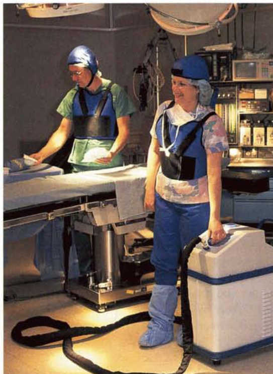
A variation of the MS patient's cool suit is the Mark I Surgical Personal Cooling System for medical personnel who must wear protective clothing in hot operating room environments.
