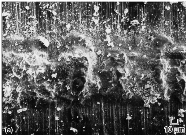
Figure 11.—Surface damages produced on both (a) Ti-48Al-2Cr-2Nb fatigue specimen and (b) superalloy contact pad. Table 2(b.2) presents the fretting conditions.
