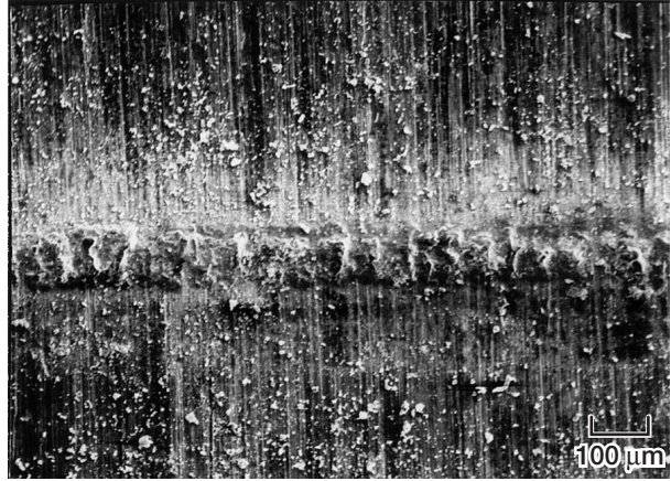
Figure 9.—Wear scar with wear debris particles produced on Ti-48Al-2Cr-2Nb fatigue specimen in contact with superalloy contact pad. Table 2(b.2) presents the fretting conditions.
