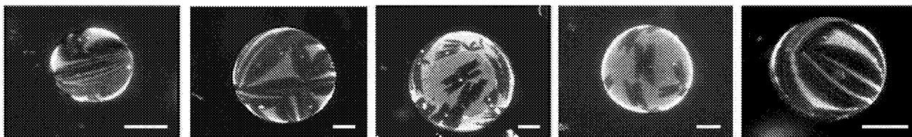
Three-dimensional reconstructed confocal microscopy images of two-dimensional streptavidin crystals (shown in black) on giant lipid bilayer vesicles. Scale bar represents 10 \mu\text{m} .
