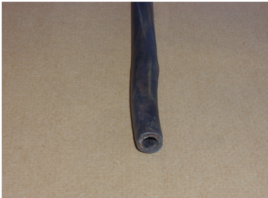
Figure 8 – Specialist Sulphur Probe Deformation/Warping
