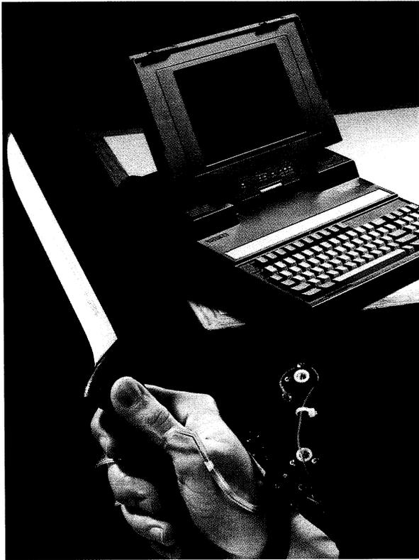
The DHM II is worn on the hand, connected to a computer that records hand motions and transmits that data as control signals to robots and other computers. It is used in such applications as enabling robotic hands to emulate human hand actions through remote operation; controlling and manipulating computer generated images in virtual reality environments; and controlling musical performances by shaping acoustical parameters in real time, on stage, in concert with musicians.
