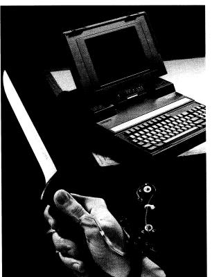
The DHM II is worn on the hand, connected to a computer that records hand motions and transmits that data as control signals to robots and other computers. It is used in such applications as enabling robotic hands to emulate human hand actions through remote operation; controlling and manipulating computer generated images in virtual reality environments; and con-
