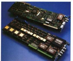
The Convolvotron consists of a two-card set designed for use with a personal computer. The system's 128 parallel processors make the Convolvotron 20 times faster than ordinary digital signal processing systems, the company states.
