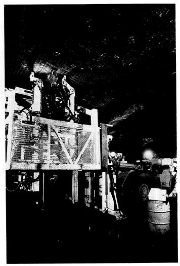
chine from a position under an already-screened area, where he is protected from rockfall; he positions the mesh, drills in a predetermined pattern, then inserts and tightens the rock bolts, handling 35 feet of screening and 18 bolts in a three-hour sequence. The system not only improves safety in a hazardous operation that costs more than a score of lives annually, it also increases productivity fourfold.
