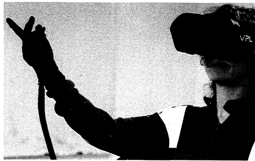
The VPL Research EyePhone is a headset in which the viewer can't see the physical world, instead sees a computer generated VR world in color and 3D. With the DataGlove, the goggled VPL engineer shown can virtually grasp and pick up objects in the VR world as if they were real.
