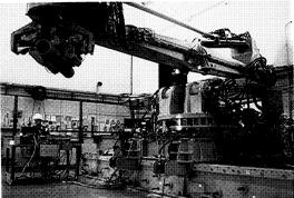
understanding with Inco Limited, Mississauga, Ontario, the world's largest nickel producer, to join in development of remotely controlled underground mining equipment, based on Canadarm technology, for improved safety and productivity in deep-Earth, hard-rock mining. ▲
