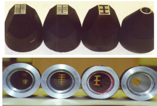
Figure 2 Photographs of subsonic 14, 10, 6 lobed and circular nozzles
