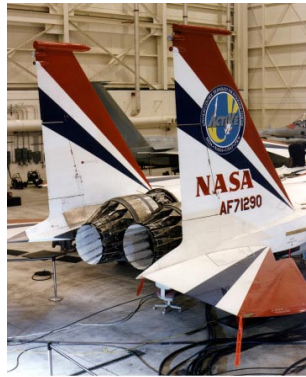
Dryden Flight Research Center EC95-43273-4 Photographed 1995 F-15 Advanced Control Technology for Integrated Vehicles (ACTIVE) showing thrust-vectoring nozzles. NASA photo
