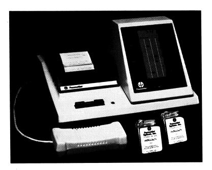
of the implantable pacemaker together with a physician's console containing the programmer and a data printer. Below, the physician is communicating with the patient's pacemaker by means of wireless telemetry signals transmitted through the communicating head held over the patient's chest.
