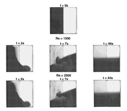
Evolution of Kelvin-Helmholtz Instability Waves During Mixing Due to Impulsive Input Velocity,  $Gr = 3.18 \times 10^6$ ,  $Re = 2 \times 10^4$ , Ar = 0.2
