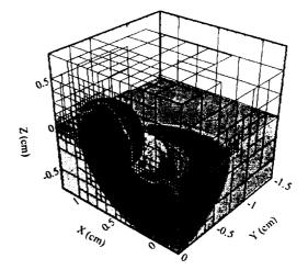
FIGURE 2. Highly oblique impact of 1/4" spherical aluminum projectile onto aluminum half-space target. Level 7 adaptive mesh (equal to 160 cells across the projectile diameter) is shown. Block outlines are shown. Color represents pressure. This calculation ran 15 times faster than a comparable resolution non-AMR run.
