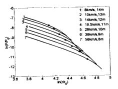
**Figure 2:** Normalized tensile pressure P at different depths, r, for sets of impact velocity U (km/s), and impactor radius  $r_0$  (m) constrained by fracture depth of Meteor Crater and dynamic tensile fracture strength of Coconino Sandstone.  $P_0$  is initial impact pressure,  $P=P_r-P_z$ , where  $P_r=P_0(r/r_0)^{-n}$ ,<sup>[8]</sup> n is function of U<sup>[9]</sup> and  $P_z$  is the lithostatic pressure. Circles represent r = 850 m and P = 40 MPa.
