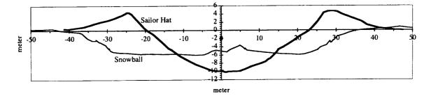
Figure 1. Comparison of crater profiles from two explosive field tests. Both tests used hemispherical charges of TNT (4.5x10<sup>8</sup> g) situated at the target surface. The Sailor Hat event was conducted in basalt, whereas Snowball was conducted in unconsolidated alluvium with the water table at a depth of approximately 7 m.
