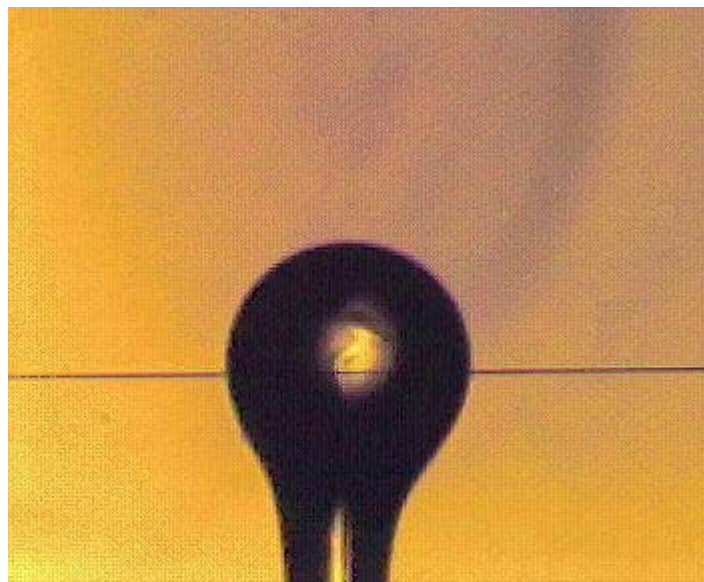
Figure 4. Photo of MOMS sensor: Fiber diameter \sim 5 \mu\text{m} and sphere diameter \sim 350 \mu\text{m} .
