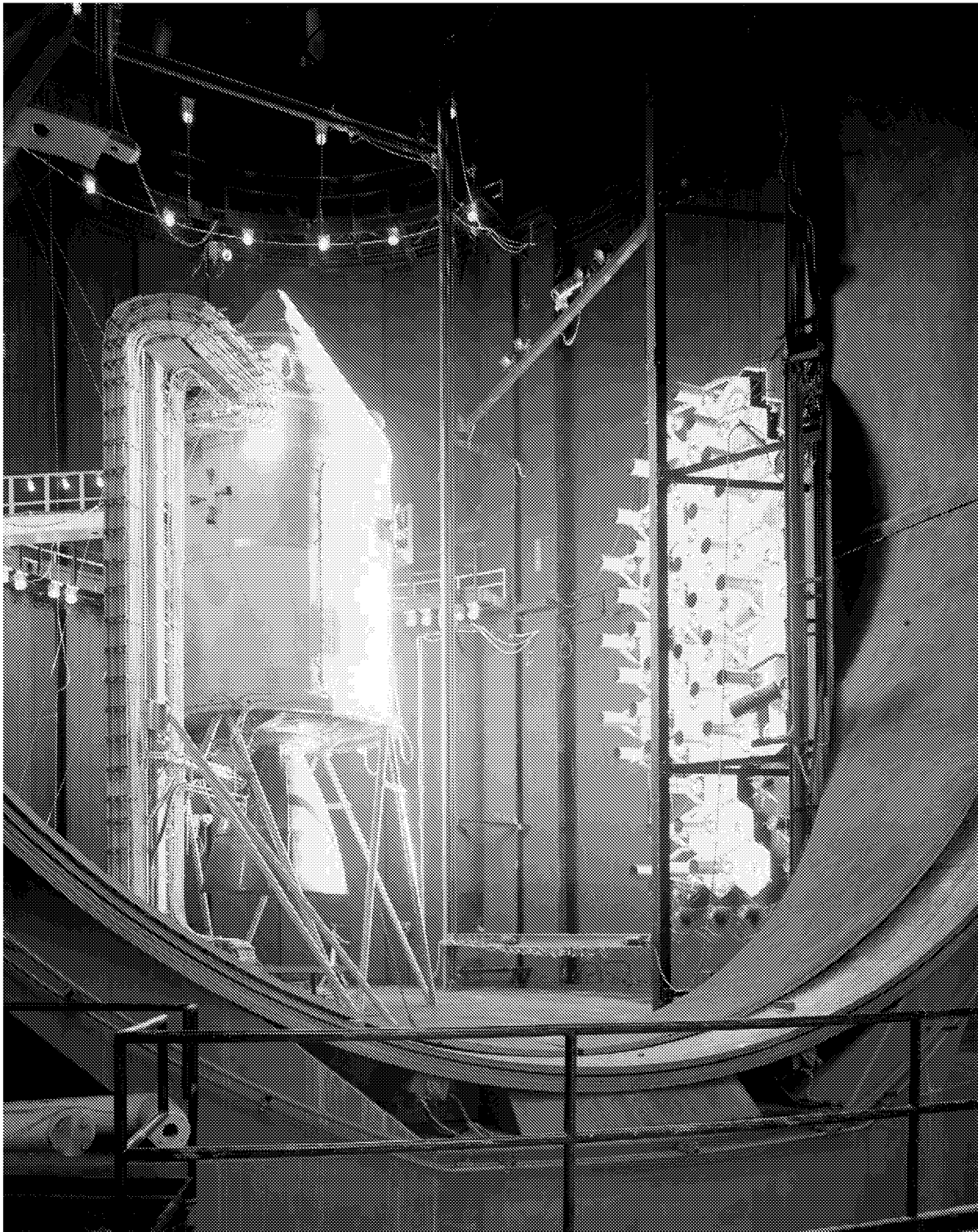
S/C 008 in Chamber A with full side-sun simulation.
