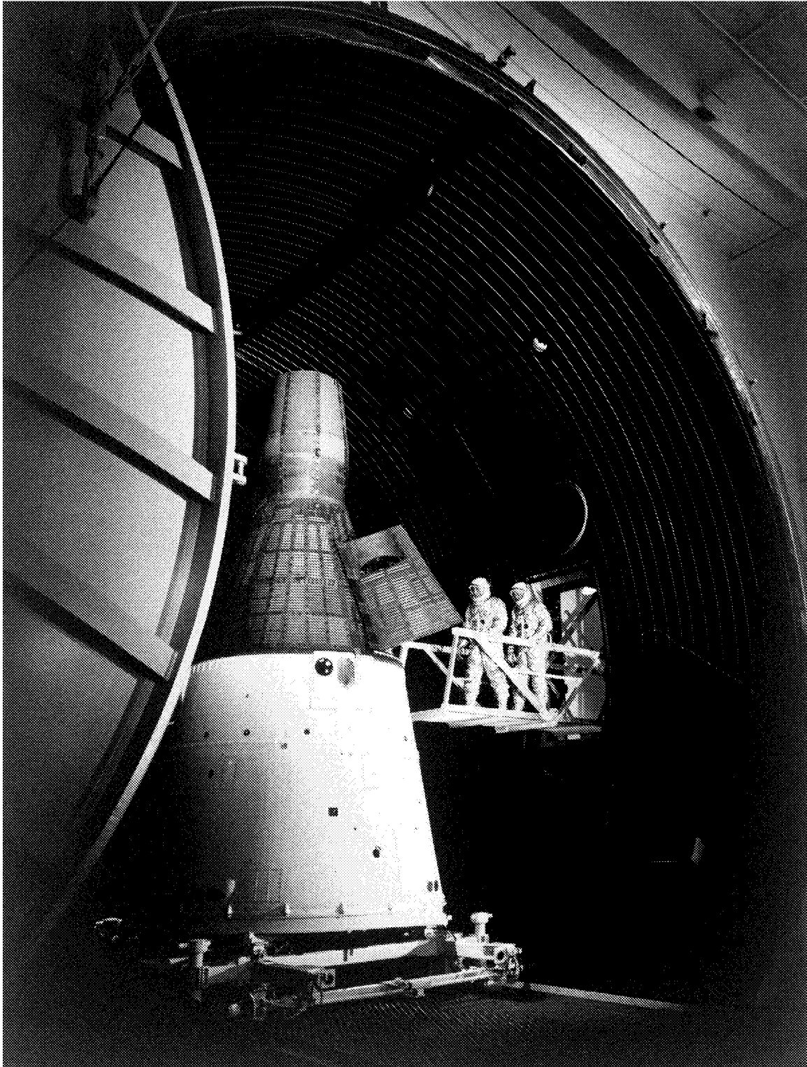
Gemini spacecraft testing at the McDonnell Aircraft Corporation 30-foot chamber.
