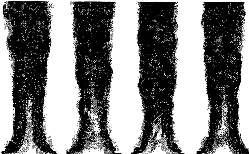
FIGURE 1. Instantaneous temperature contours of a one meter diameter methane fire at different times (increasing left to right), illustrating the puffing behavior of the pool fire.
