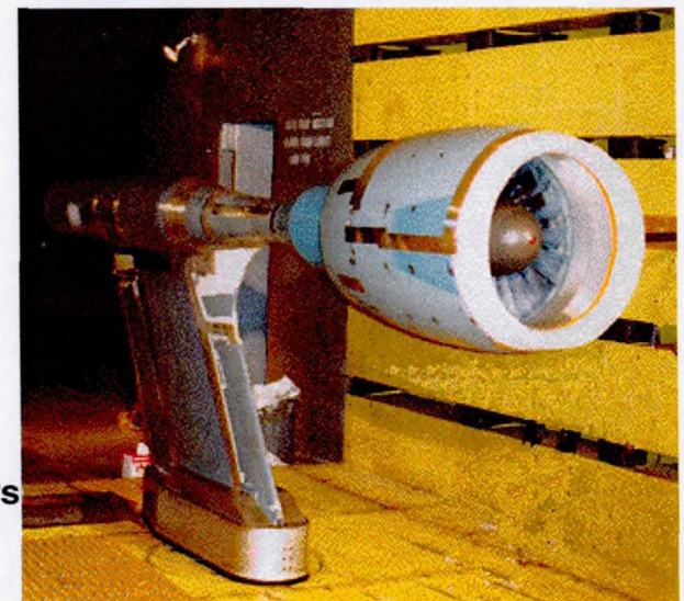
Northrop Grumman Hybrid Active/Passive Liner Installed in the NASA ADP Fan Rig at the NASA LeRC 9'x15' Wind Tunnel
