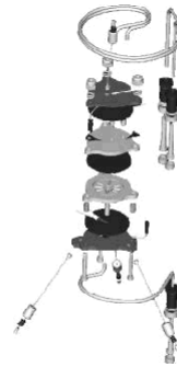
Figure 3. Exploded view of an electrolyzer assembly.
