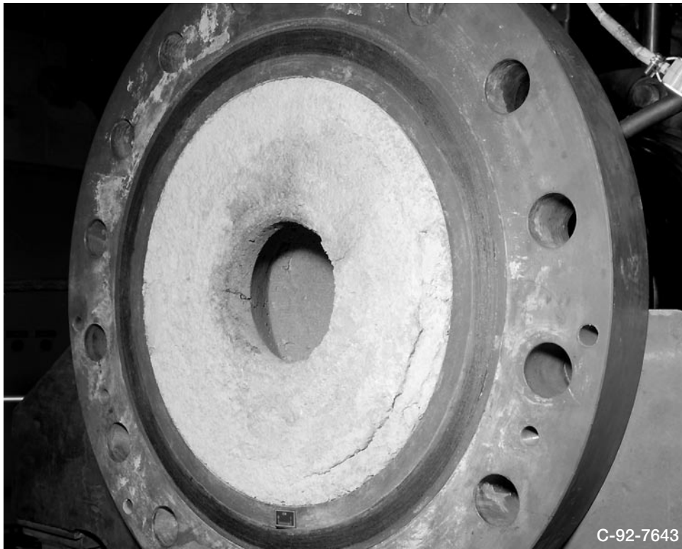
Figure 3.—Rich burner module with castable liner.
