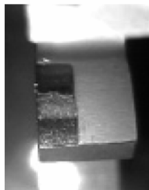
Figure 3.33.—Damage progression of driver/driven tooth 3 for experiment 19
