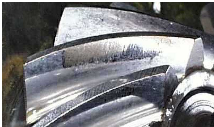
Figure 4.9.—Damage to left pinion teeth during bevel test 2.
