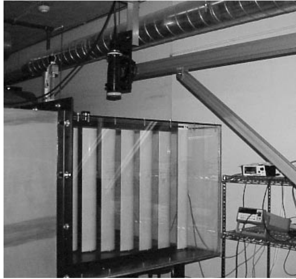
Figure 17: Photograph of LDV fiber-optic element and photo-multiplier assembly positioned on 2-D traverse and extending over cascade test section.
