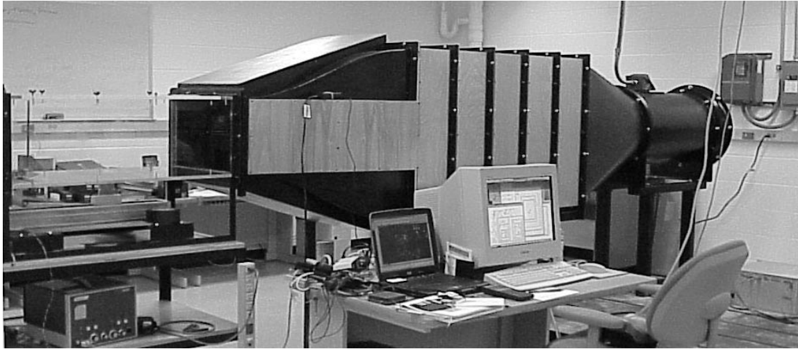
Figure 15: Photograph of new, general purpose wind tunnel that was built to develop new moving wake concept. Test section dimensions are 12 \times 18 in. cross-section, by 36 in. long. Maximum velocity is 50 m/s.
