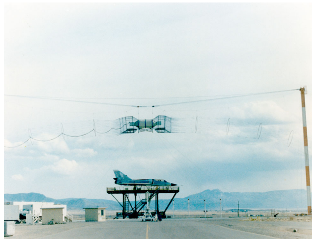
NASA 816 during nuclear electromagnetic pulse simulation testing at Kirtland Air Force Base. Photograph on left shows aircraft being hoisted to test platform and one on right shows aircraft in place for tests.
