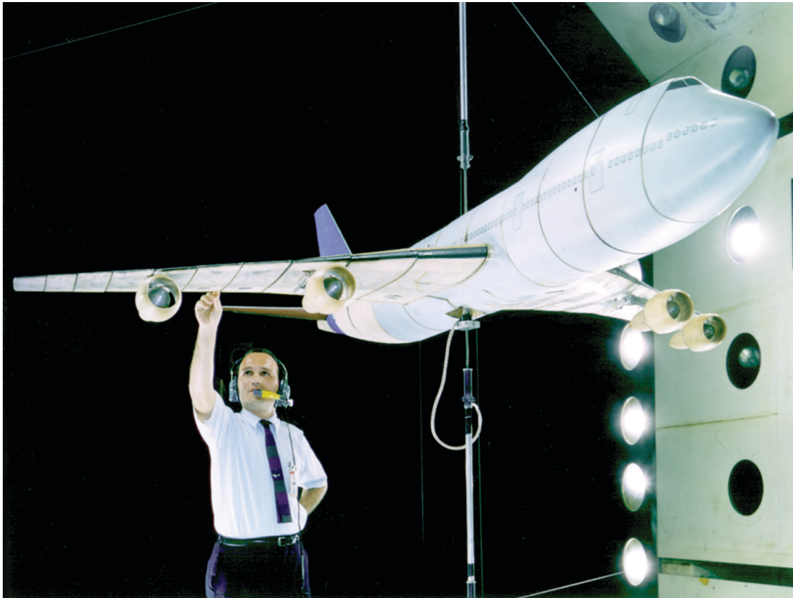
Researcher Irving Abel with Boeing 747 flutter model.
