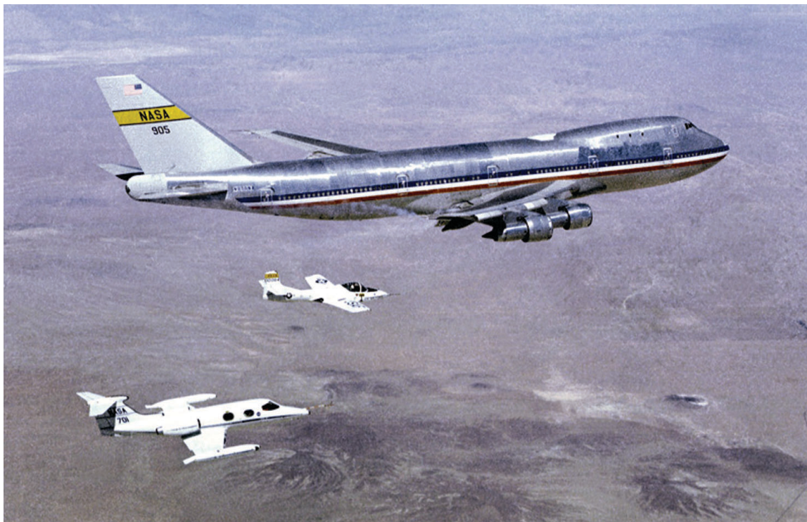
NASA conducting flight assessments of wake-alleviation concepts at Dryden with NASA Boeing 747, T-37, and Learjet aircraft.
