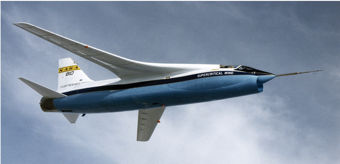
F-8 supercritical wing test-bed aircraft in flight with an area-ruled fuselage and underwing leading-edge vortex generators.
