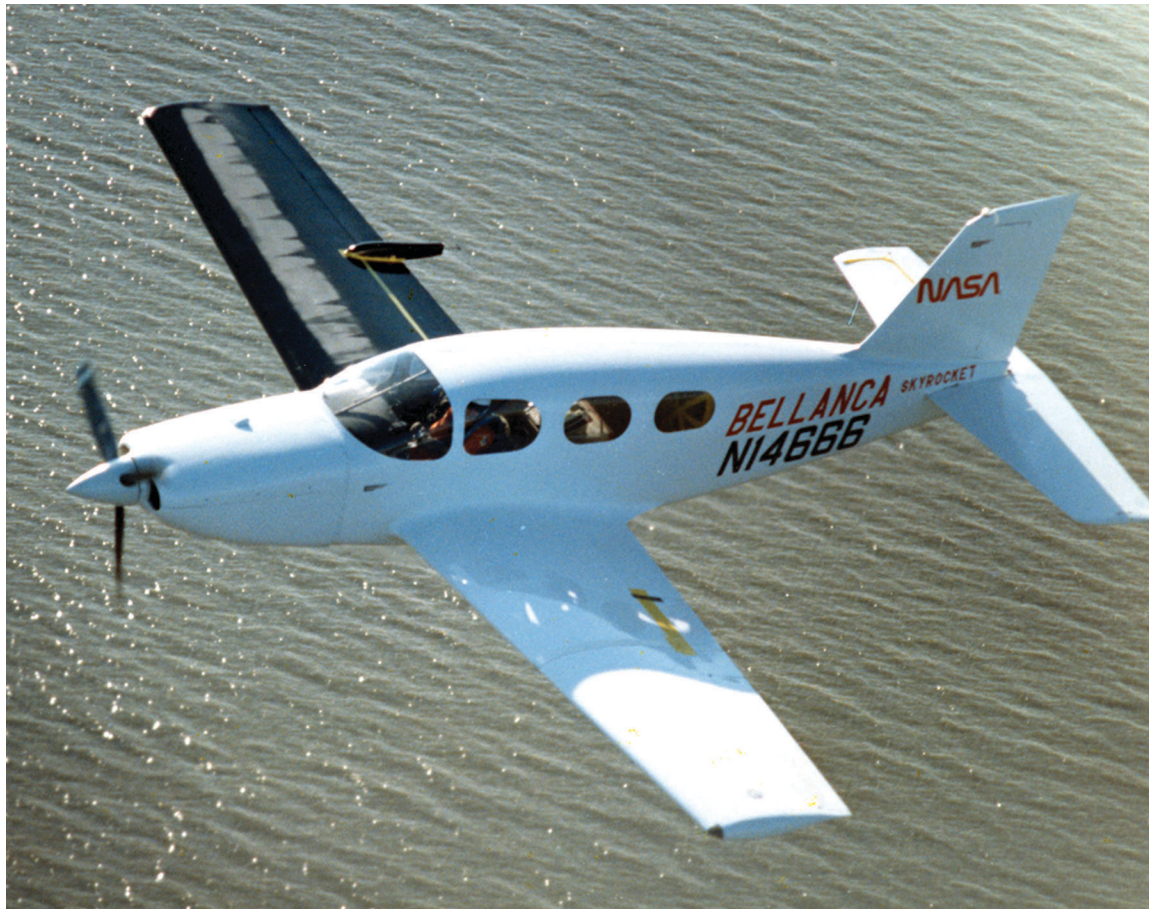
Sublimating chemicals on right wing of Bellanca Skyrocket indicating large extent of natural laminar flow during Langley flight tests.
