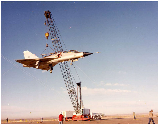
NASA 816 during nuclear electromagnetic pulse simulation testing at Kirtland Air Force Base. Photograph on left shows aircraft being hoisted to test platform and one on right shows aircraft in place for tests.
