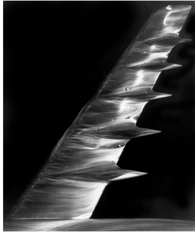
Oil flow visualization of model wing with 35° sweepback at Mach number of 0.90 and angle of attack of 4° (flow is left to right). A significant amount of unacceptable flow separation is evident for basic wing (left) on rearward part of wing; the addition of antishock bodies (right) greatly reduces separation.
