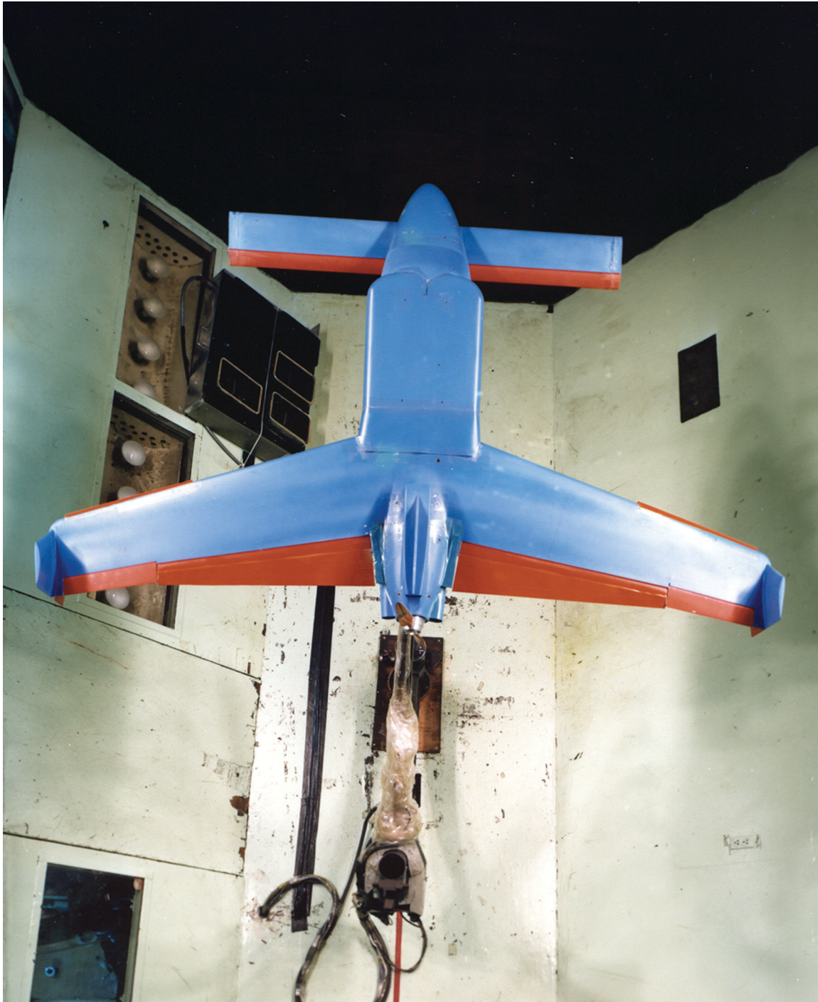
Model of OMAC 300 in Langley 12-Foot Low-Speed Tunnel. Note leading-edge droop and extended chord of wing trailing-edge flap.
