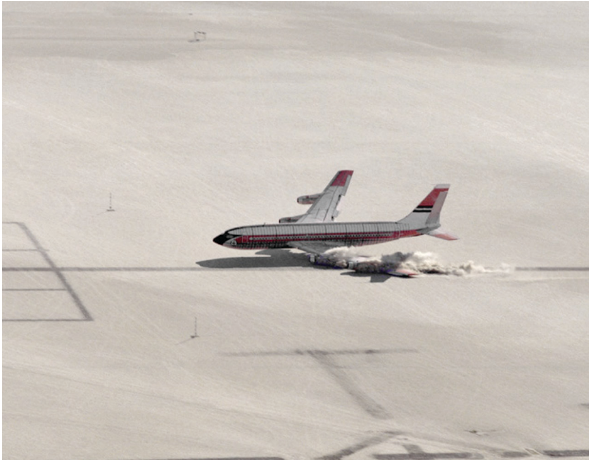
Impact of Boeing 720 during NASA and FAA Controlled Impact Dynamics Program in 1984.
