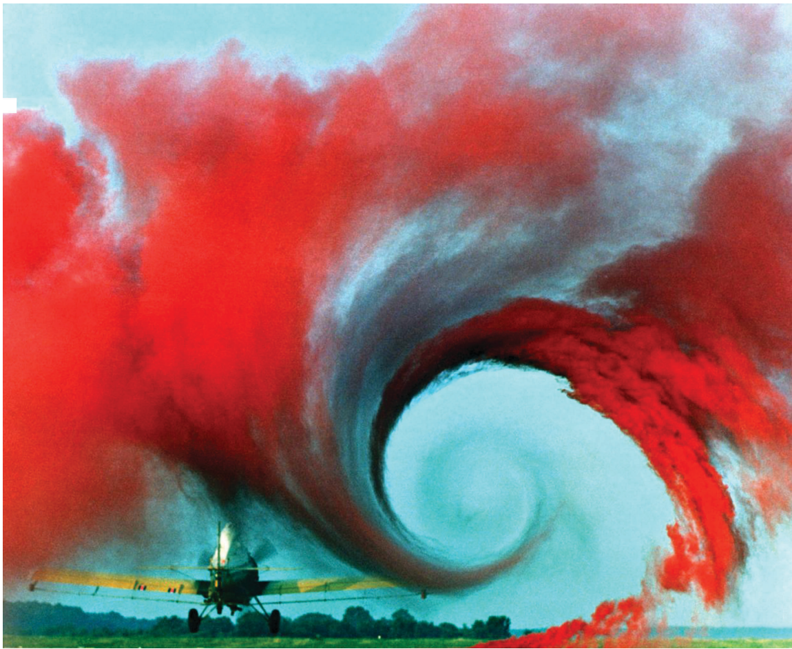
Langley pilot Philip Brown flies Thrush Commander over smoke injection system for visualization of wake of aircraft.
