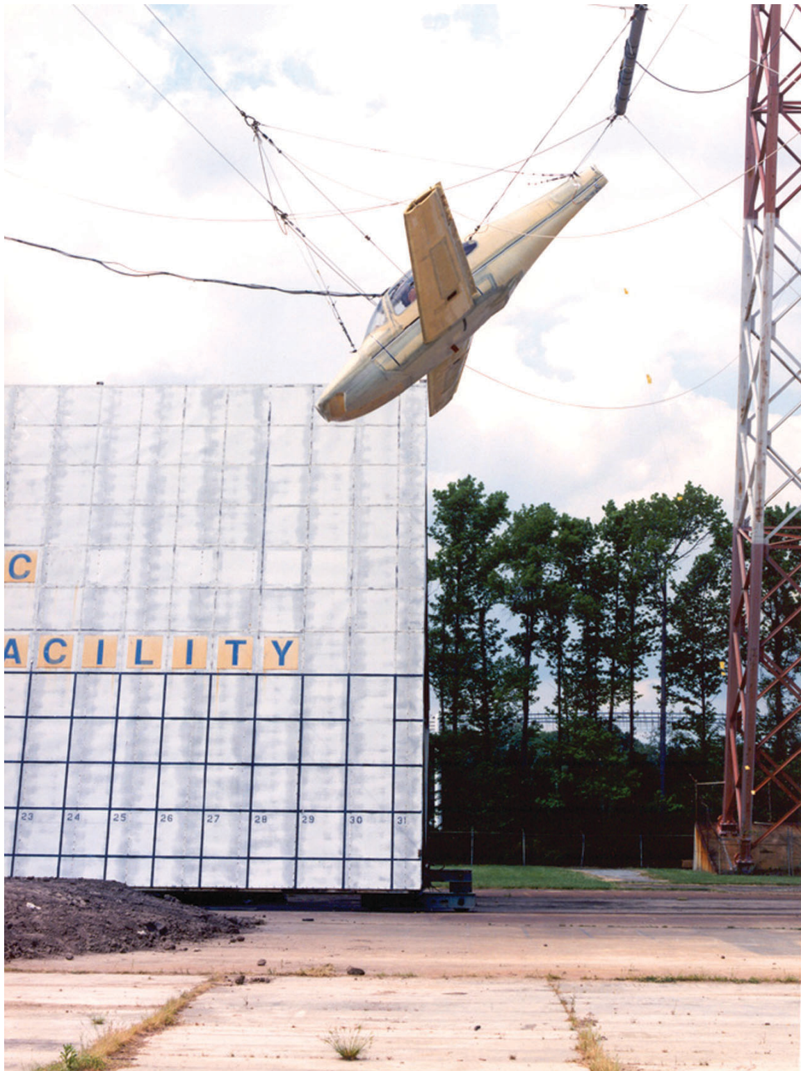
Test aircraft suspended for crash test in Langley and Terry Engineering investigation of improved crashworthiness. Note soil spread over impact surface for soft soil test.
