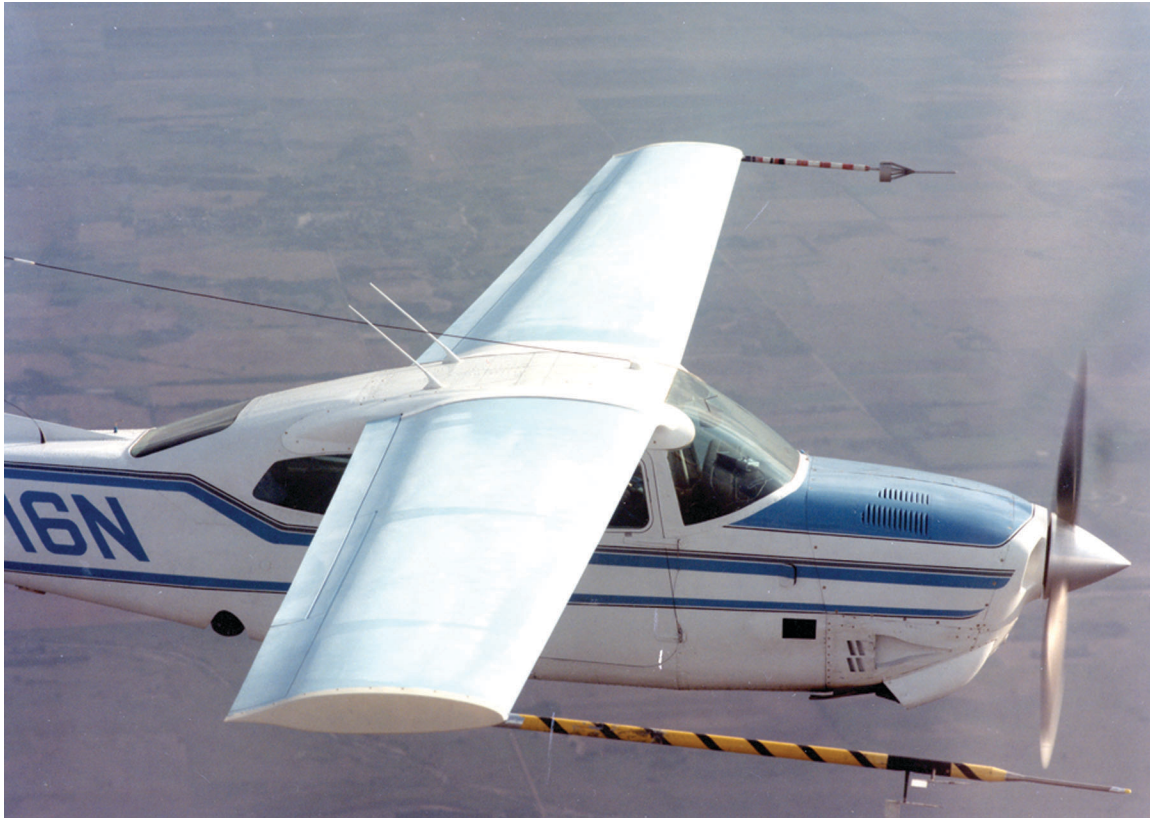
Chemical sublimation patterns on wing of modified Cessna Centurion showing large areas of laminar flow at 125 knots in NASA-Cessna flight tests. Note wedges in pattern caused by intentional trips.
