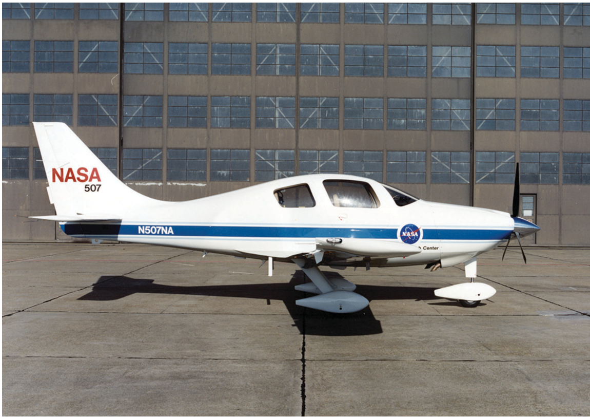
NASA's Columbia 300 research aircraft showing shape of natural laminar flow airfoil used by the wing.
