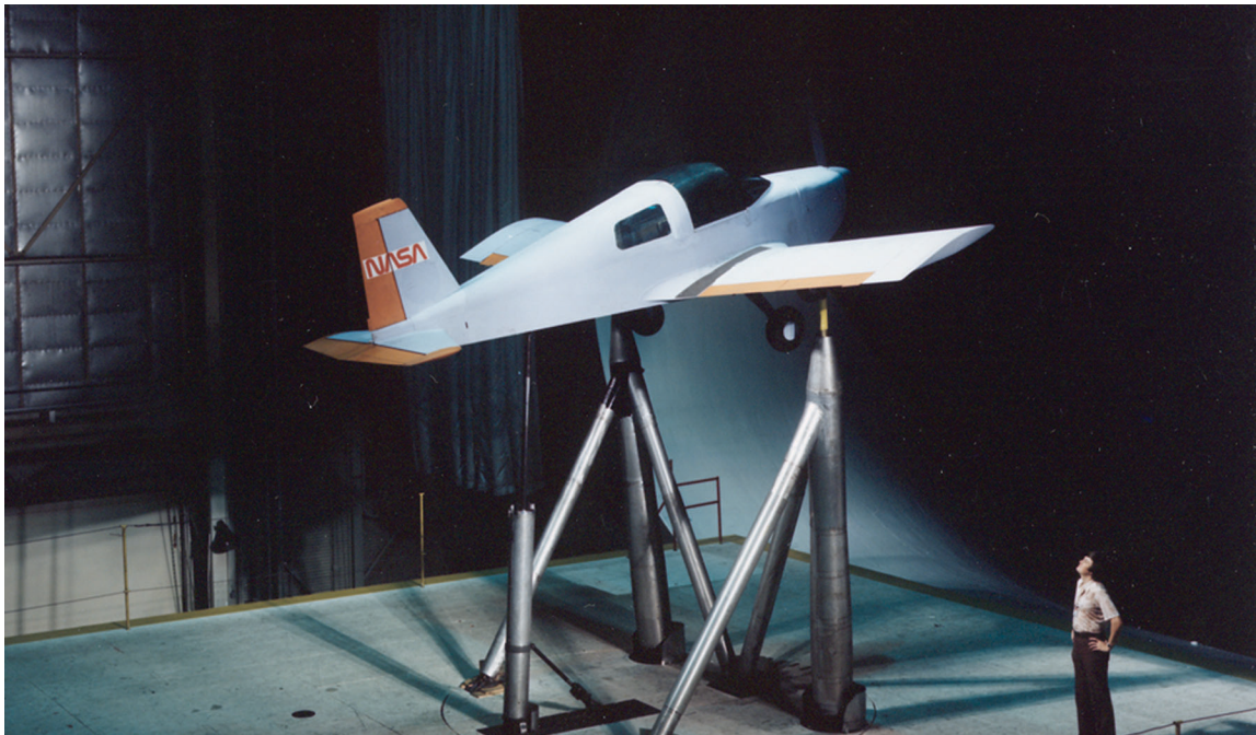
Researcher Dale Satran inspecting full-scale powered model of AA-1 research aircraft during tests of automatic stall-prevention concepts in Langley 30- by 60-Foot (Full-Scale) Tunnel.
