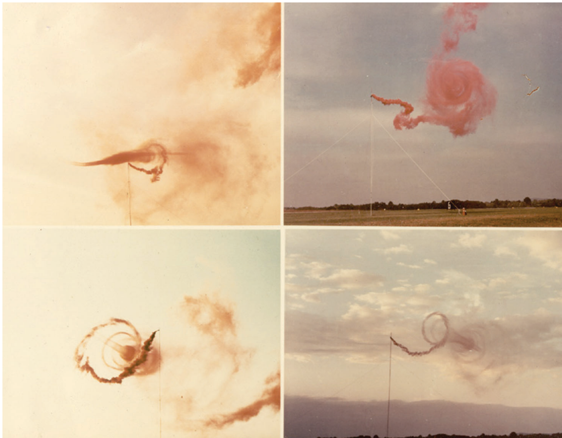
In 1970 NASA Marshall Space Flight Center conducted flyby studies of vortex-wake behavior with smoke ejected from tower entrained into vortex to permit visualization of character and persistence of vortex.
