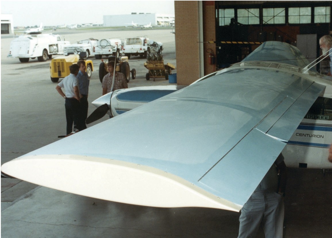
Postflight inspection of Centurion still displays extent of laminar flow exhibited in-flight at test condition.
