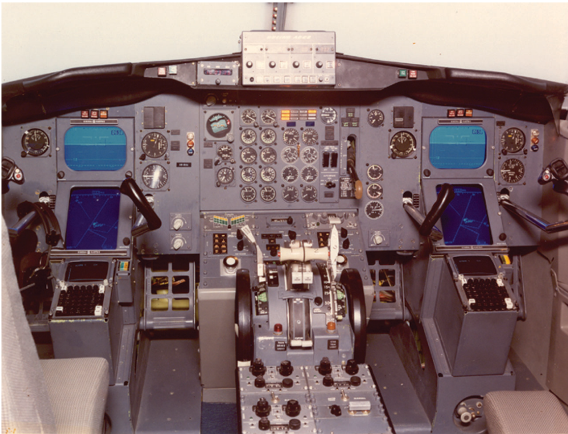
Research deck (aft cockpit) of TSRV configured with CRT displays.
