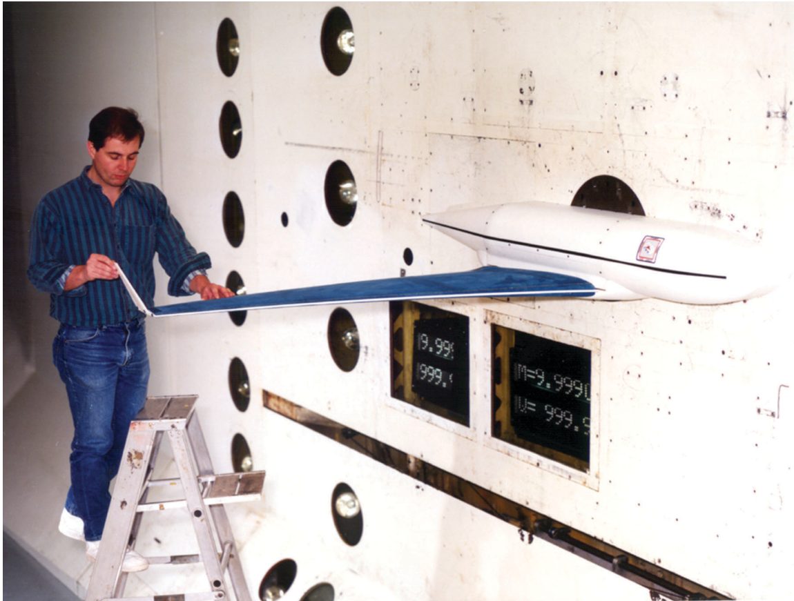
Donald Keller with Gulfstream V model during winglet flutter investigation.
