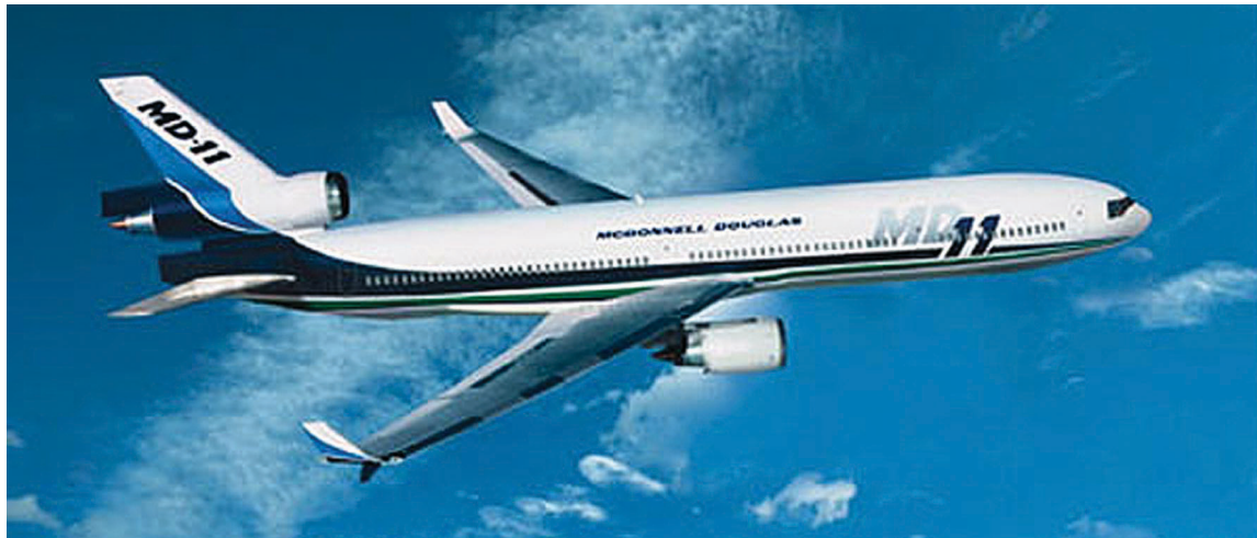
McDonnell Douglas built on development experience gained in NASA ACEE Program to design winglets for the MD-11.
