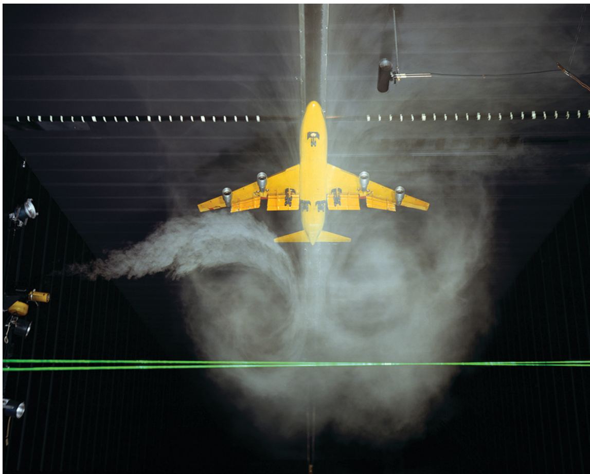
Laser beams used to measure air velocities at specific points in wake for Boeing 747 model in VRF.
