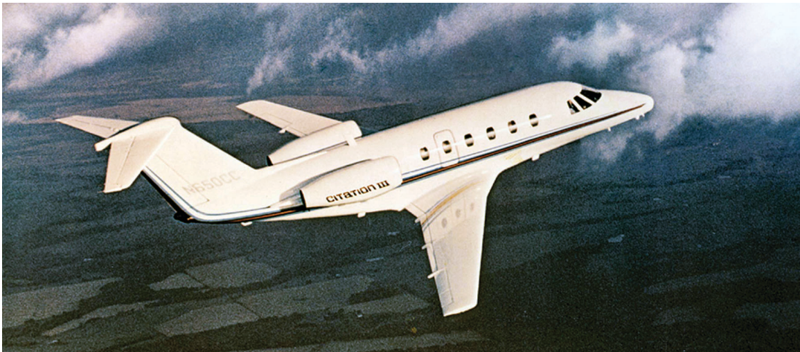
Cessna Citation III was the first application of supercritical technology to production aircraft in the U.S.
