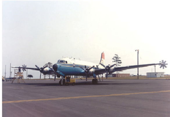
Langley's evaluation of spline device on C-54. Top photographs show VRF results for basic (left) and modified model, showing diffuse wake with spline. Lower photographs show installation of splines on full-scale aircraft.
