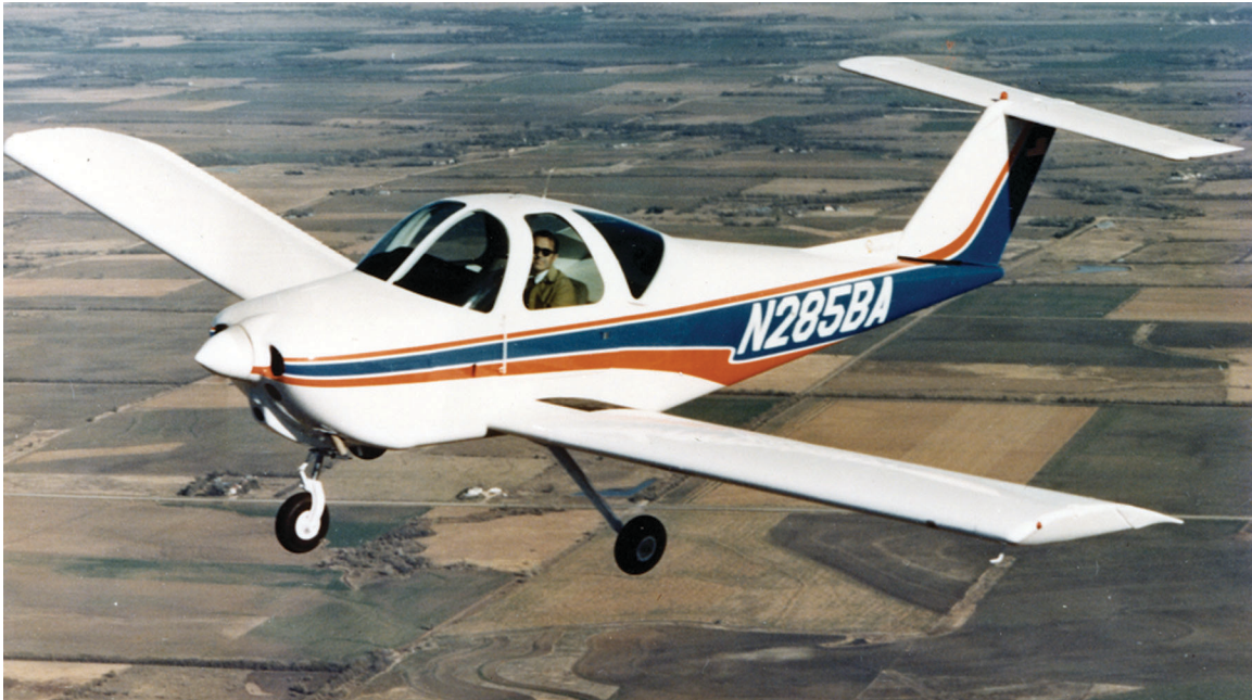
Beechcraft Model 77 Skipper was one of the first applications of GAW(1) airfoil in 1977.
