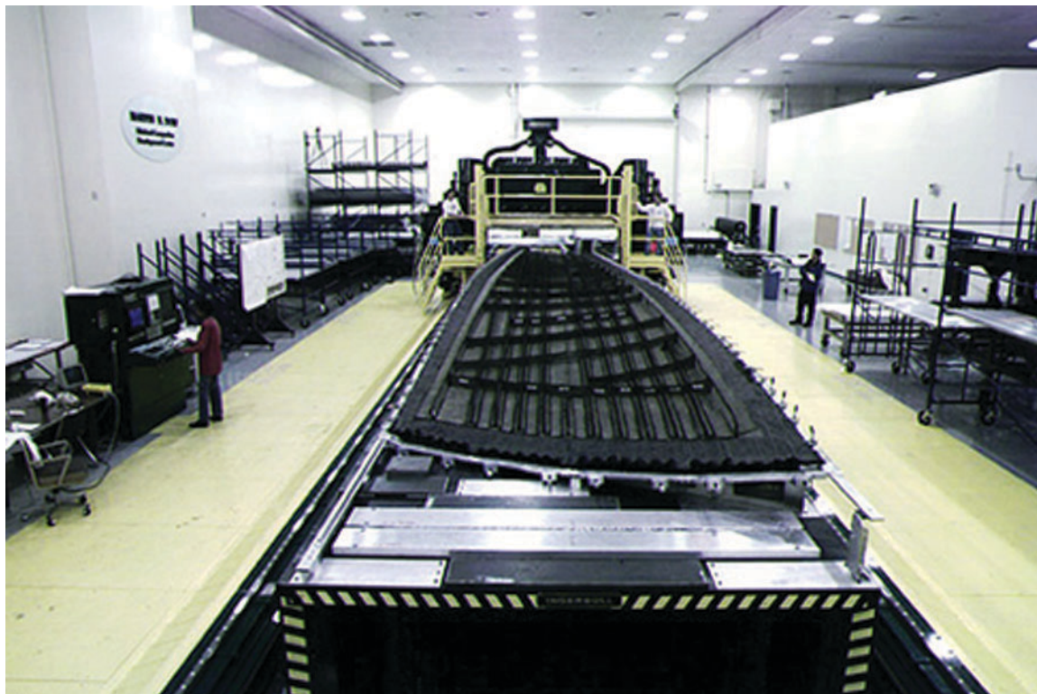
Lower-stitched wing cover for 42-ft-span structural test wing.
