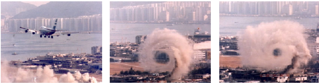
Sequence of photographs of Boeing 747 on landing approach as industrial smoke dramatically defines one of trailing vortices. Photo ©Bob Stoyles.
