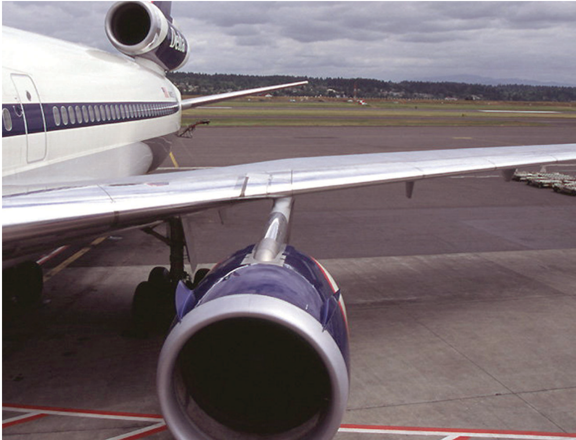
MD-11 pylon fairing retrofitted to MD-11 fleet. Photograph ©Chris Coduto.
