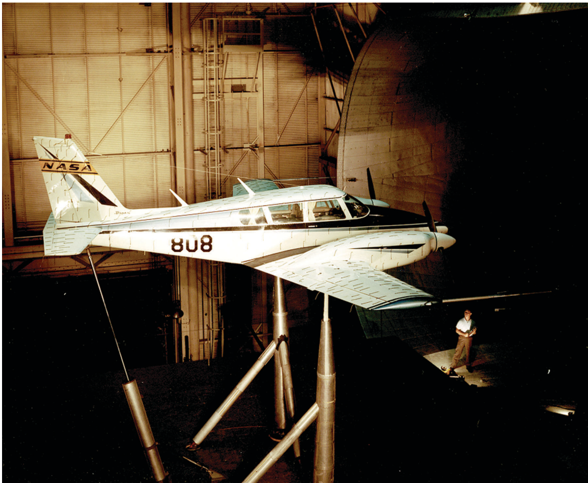
Piper PA-30 Twin Comanche aircraft mounted in Langley 30- by 60-Foot (Full-Scale) Tunnel for investigation of power-on stall characteristics.
