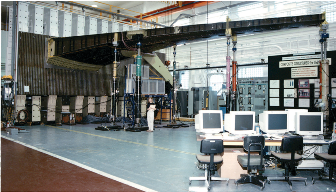
Pretest photograph of 42-ft-span wing structure at Langley.
