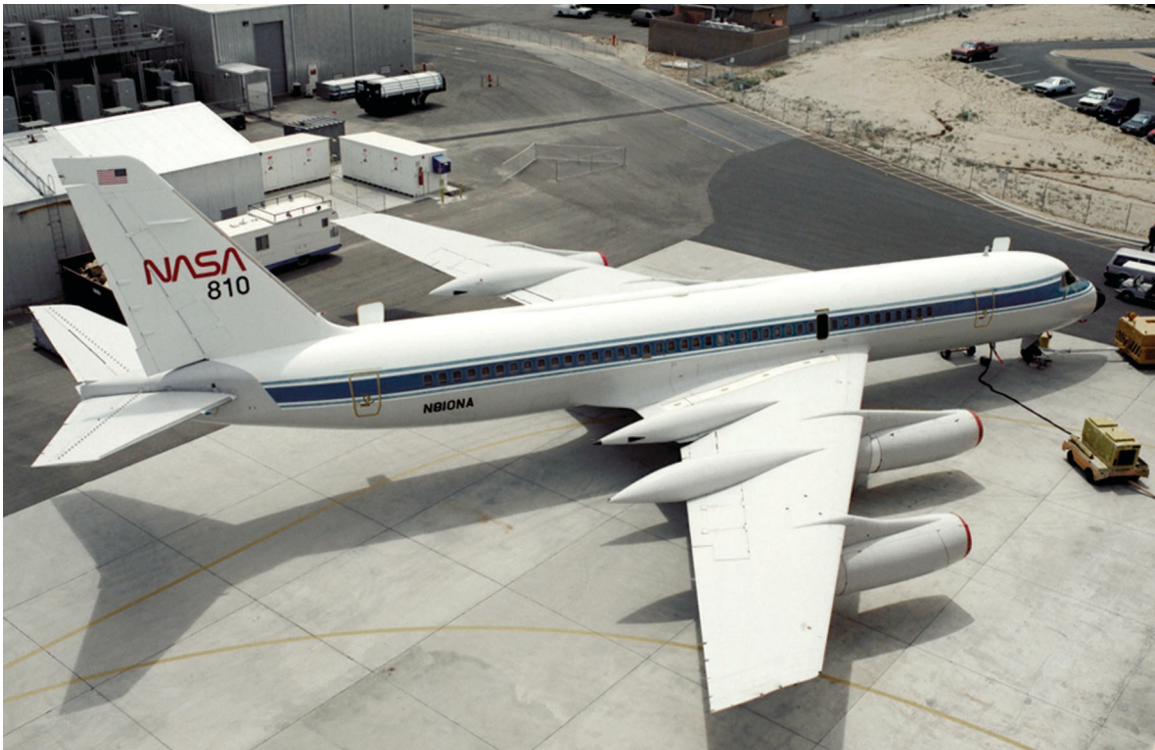
NASA's Convair 990 aircraft in 1992. Note antishock bodies on wing.
