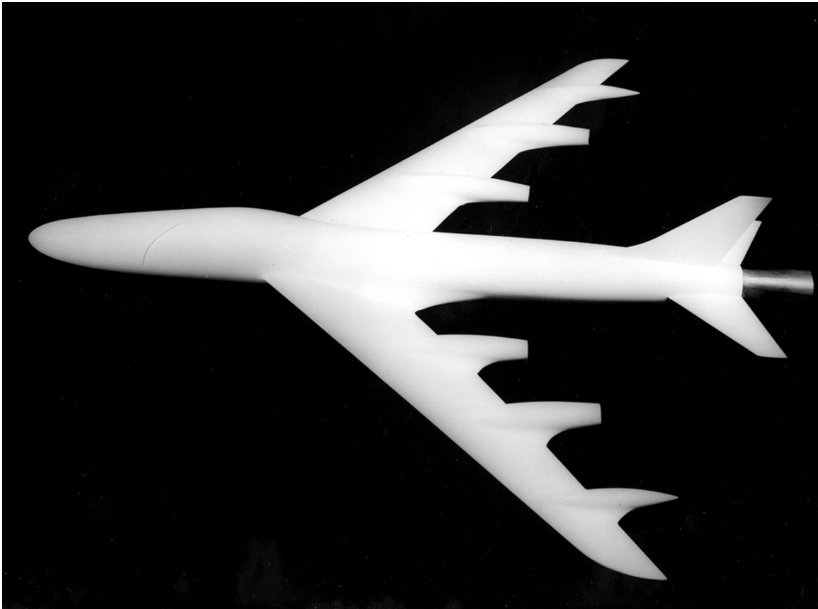
Wind-tunnel research model in Langley 8-Foot Transonic Pressure Tunnel showing upper forward fuselage fairing and antishock bodies on wing.
