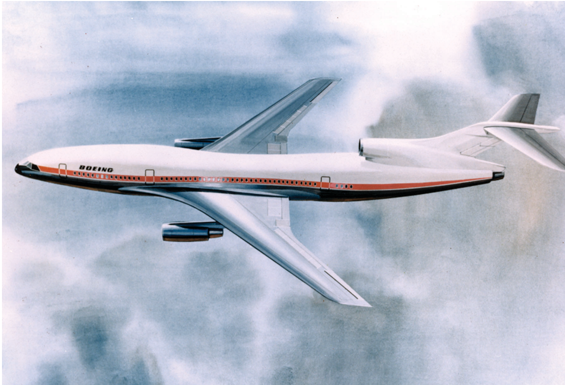
Boeing configuration in ATT studies included area-ruled fuselage.
