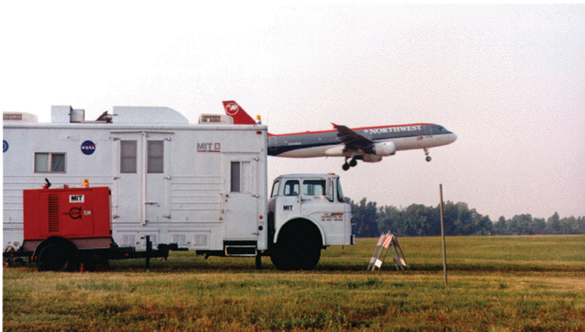
MIT Lincoln Laboratory continuous wave lidar at Memphis for wake measurements in 1994.
