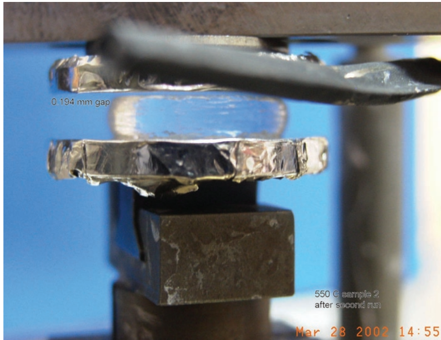
Figure 7. DMTA test fixture for parallel plate viscosity measurements.
