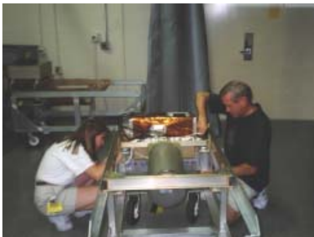
Fig. 13 Aircraft shield materials experiment rack being prepared for ER-2 flight.
