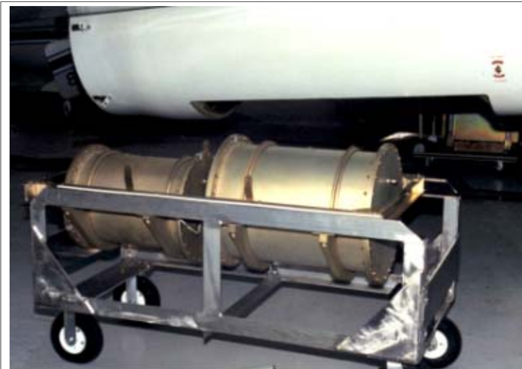
Photograph 6. Pod Rack on Ground Support Stand
