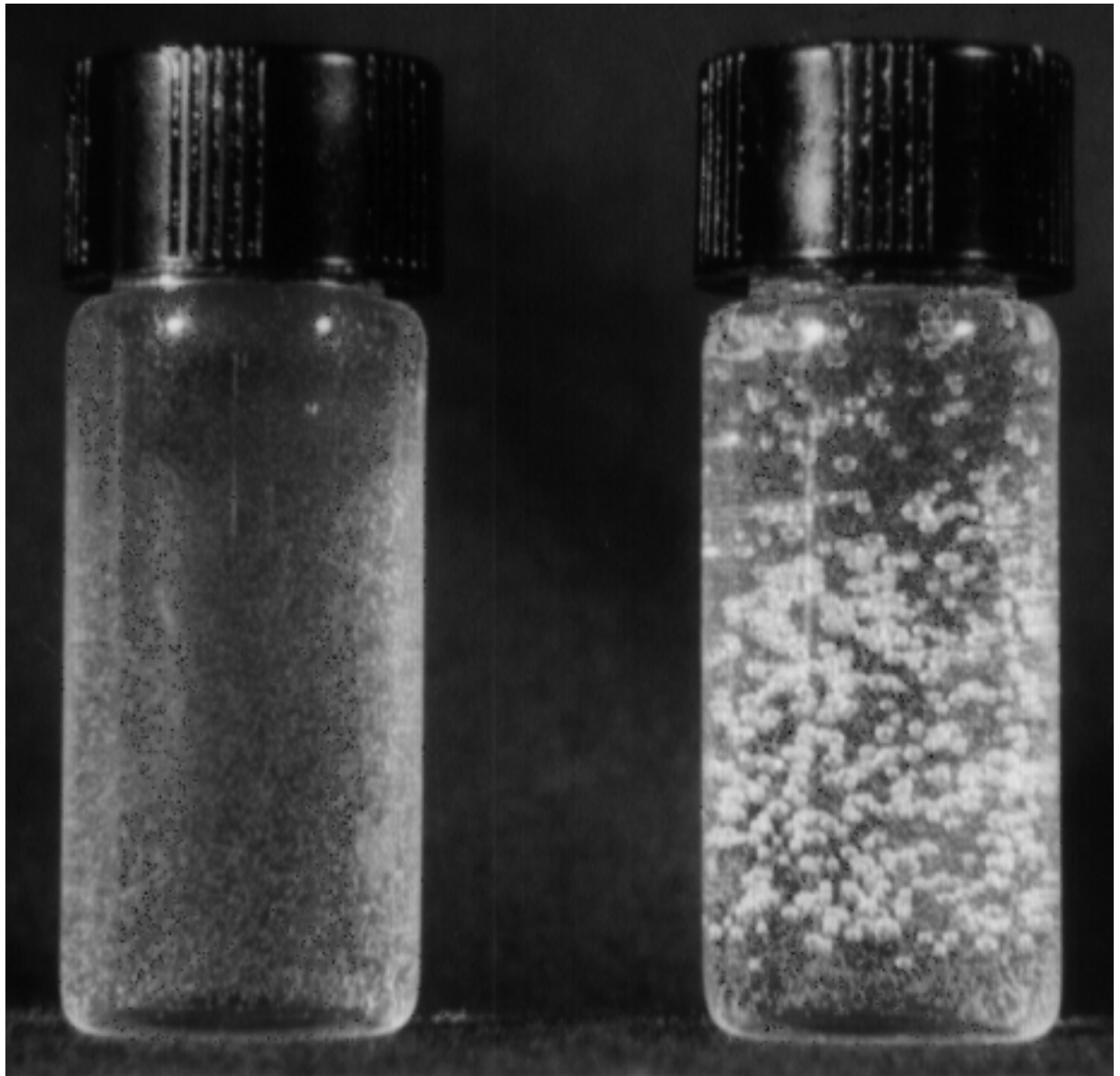
Figure 1. Superheated drop detectors before and after irradiation.
