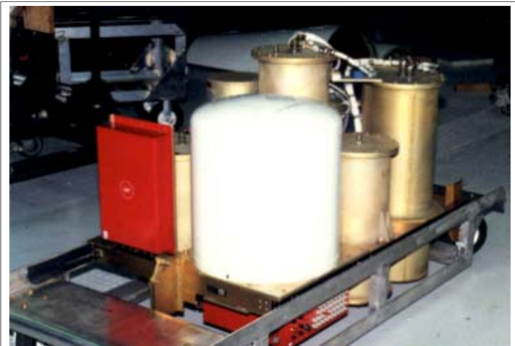
Photograph 3. Q-Bay Rack on Ground Support Stand
