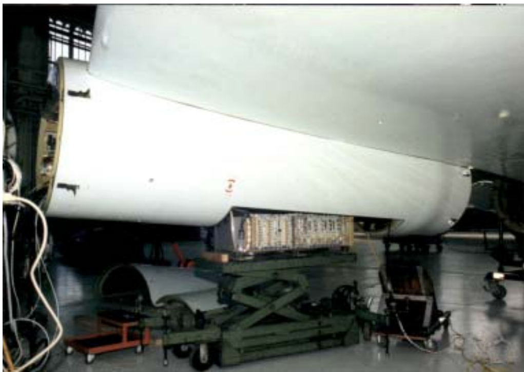
Photograph 9. Right Pod Mid-Body Electronics Installed in the ER-2
