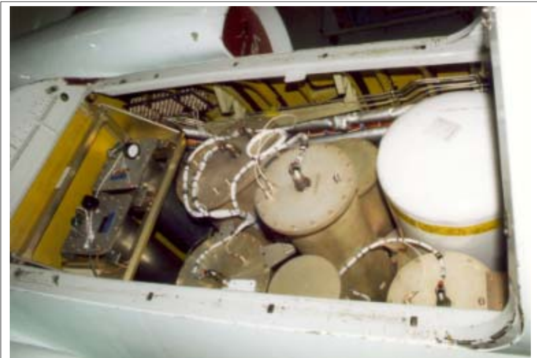
Photograph 4. Q-Bay Rack Installed in the ER-2 (Top View)
