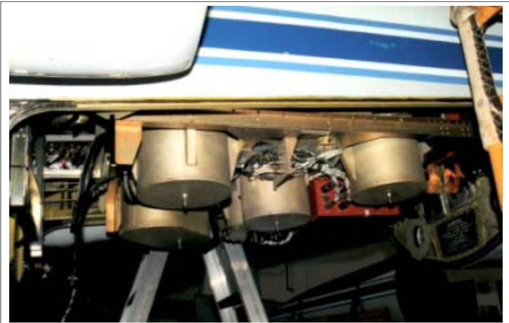
Photograph 5. Q-Bay Rack Installed in the ER-2 (Bottom View)
