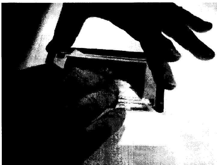
Figure 12. Manual alignment of piezoceramic fiber sheet on bottom electrode pattern.
