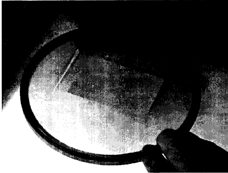
Figure 3. Removal of piezoceramic fiber sheet from dicing saw grip ring.
