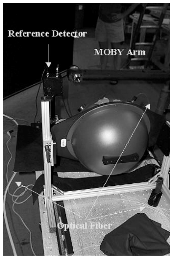
Figure 5.10: Schematic of experimental setup at the MOBY field site at the University of Hawaii Marine Center, Honolulu, Hawaii. (a) Exterior setup showing location of lasers and calibration tent. (b) experimental setup in the calibration tent for measuring the ISS radiance with a collector on the middle MOBY arm.
