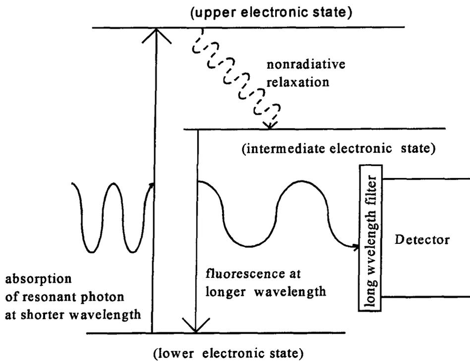
Figure 2. Illustration of Physical Principles
