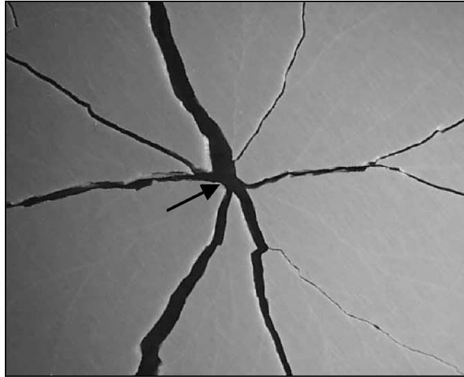
Figure 19.—Typical pattern of crack branching for AS800 silicon nitride disk impacted by 1.59-mm-diameter steel ball projectile. Arrow indicates failure origin.
