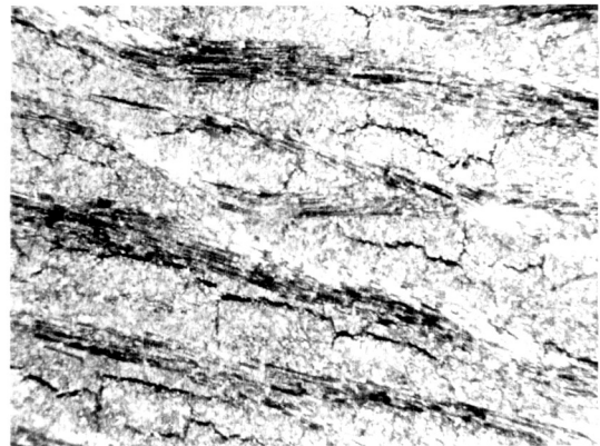
b. Microscopic View of Cracks on Outer Surface (Crack orientations are anisotropic)
