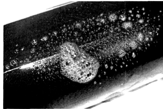
a. A Plaid Pattern like Bubbling on Outer Surface during the Leak Test
