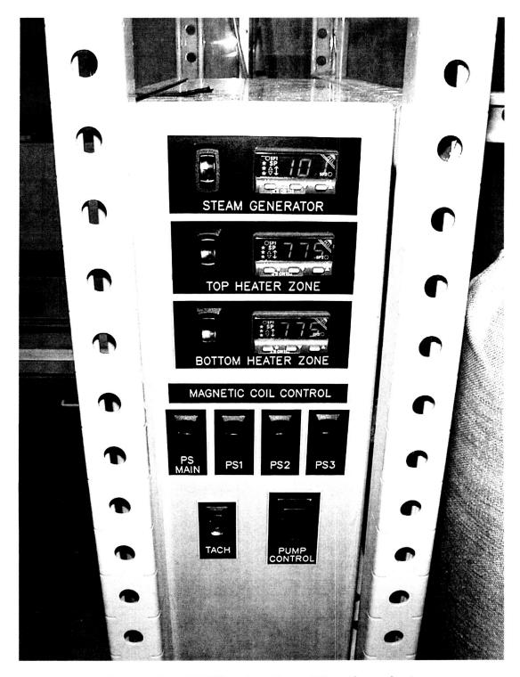
Figure 8.3. MAG Electrical Control Box (front view).
