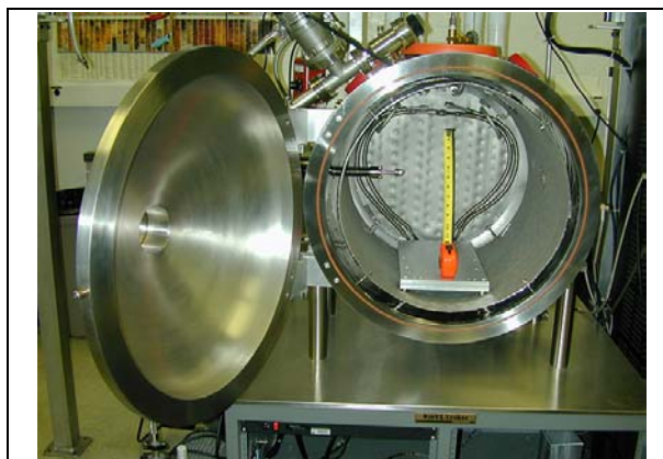
Figure 2: Cryo-shrouded vacuum chamber located the JPL's Extraterrestrial Material Simulation Laboratory.
