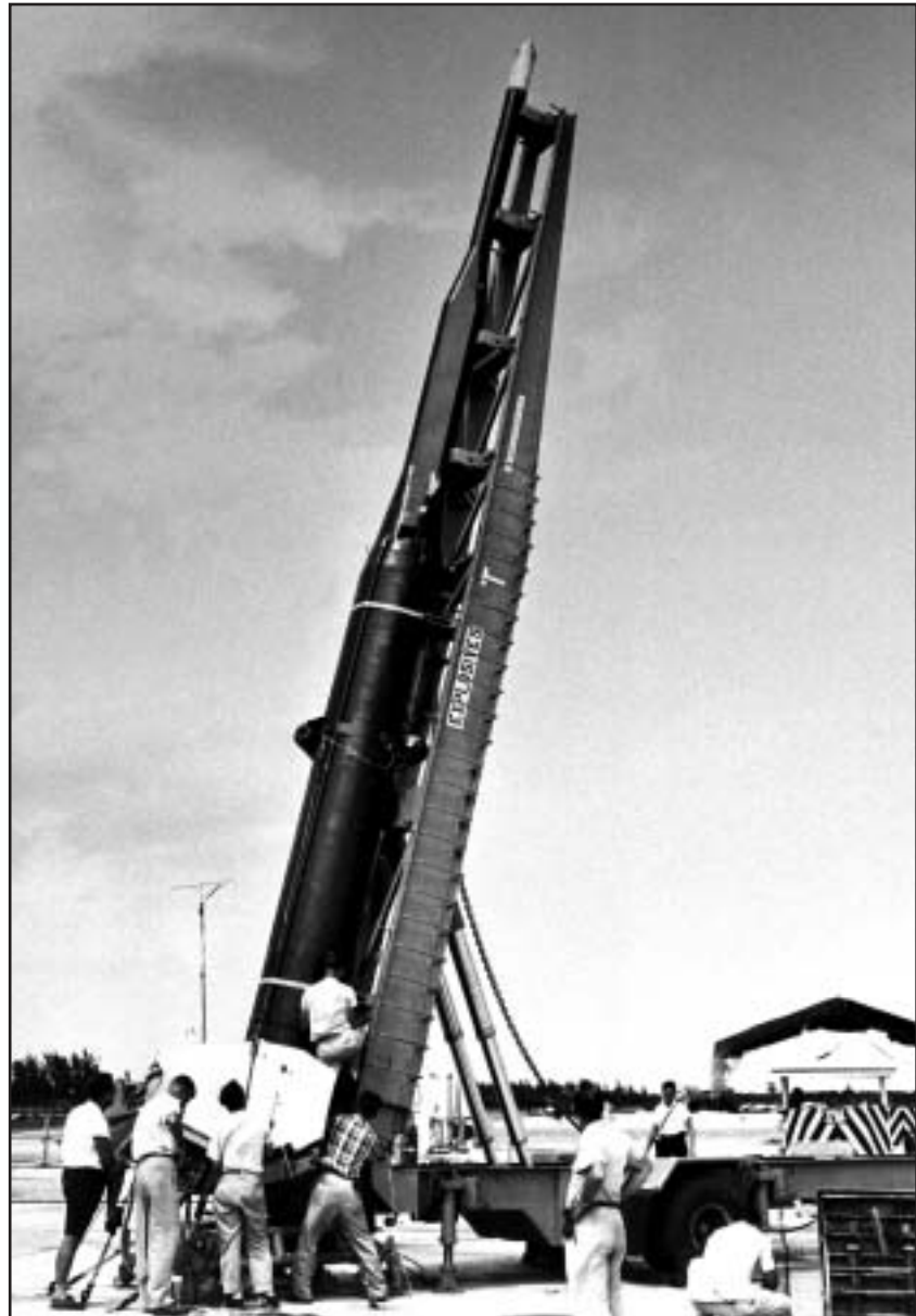
The X-17 used solid rocket motors to carry reentry vehicles to altitude. The original program objectives included reentry speeds of Mach 15 and Reynolds Numbers as high as 24 million. (U.S. Air Force via the Jay Miller Collection)
