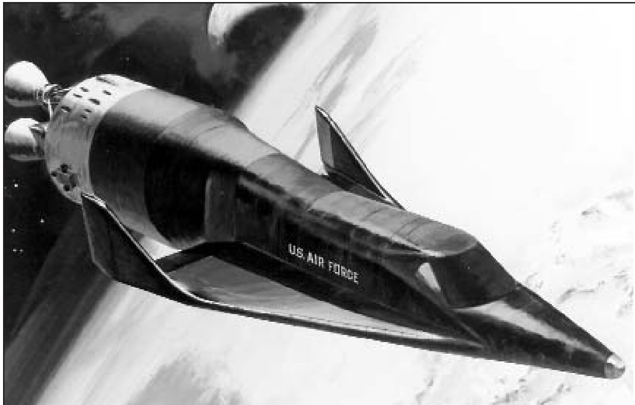
The X-20 Dyna-Soar was cancelled prior to the first flight vehicle being completed. The initial objective was to launch the Dyna-Soar on a Titan III booster to fill both experimental and, possibly, operational roles. (Boeing via the Dennis R. Jenkins Collection)
