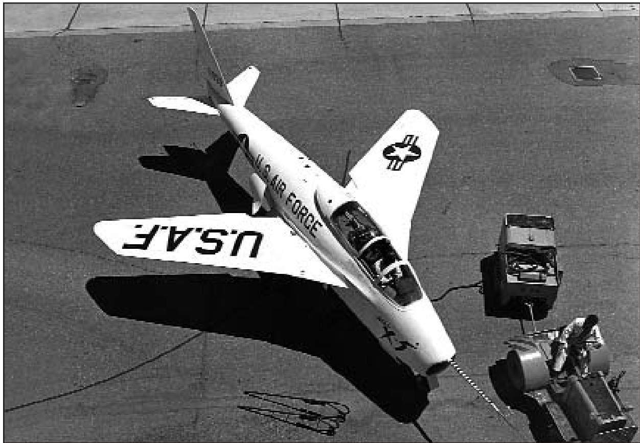
The X-5s were the first high-performance variable-geometry wing aircraft to fly. The aircraft exhibited viscous spinning tendencies, but nevertheless accomplished all of the research goals originally envisioned. (Bell Aircraft via the Jay Miller Collection)
