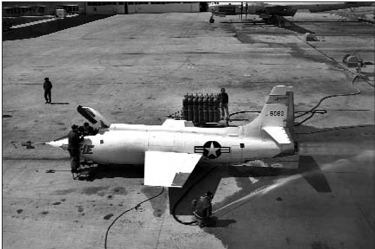
The X-1E was modified from the second of the original first generation X-1 aircraft, and is shown here conducting a ground engine run at the Flight Research Center sometime during 1956. (Tony Landis Collection)
