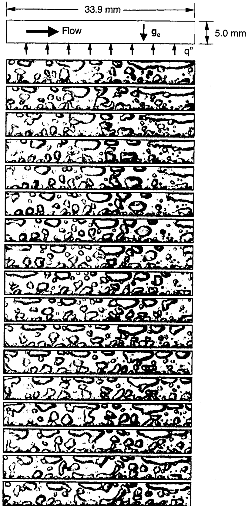
Fig. 3.3 Sequential images of vapor layer at \theta = 0^\circ and U = 0.1 m/s.
