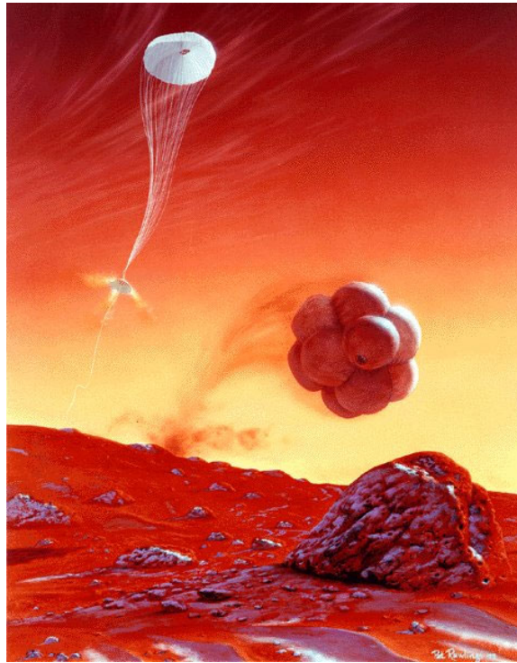
Figure 2. JPL artist depiction of Mars Pathfinder bouncing across the surface of Mars inside air bag landing system.
