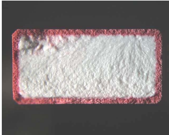
Figure 9.—Typical fracture surface of a ‘fortified’ Pyroceram specimen tested in slow crack growth testing in flexure in room-temperature distilled water. ‘Fortified’ layer is seen outside of the specimen as a red band revealed through dye penetrant.
