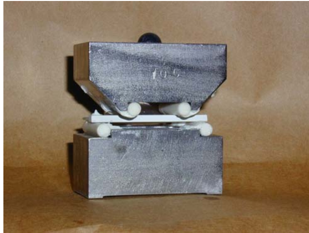
Figure 1.—Four-point flexure test fixture with a test specimen placed, used in flexure strength and slow crack growth (“dynamic fatigue”) testing for Pyroceram at ambient temperature.
