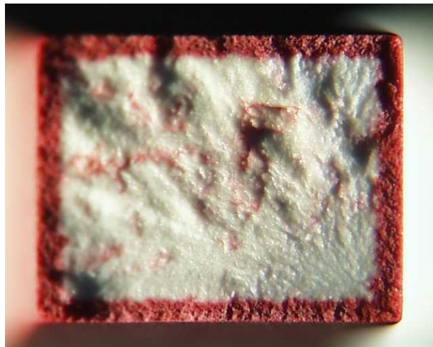
Figure 16.—A typical fracture surface of a 'fortified' test specimen in tension, showing fracture origin and 'fortified' layer. The 'fortified' layer is seen outside of the specimen as a red band revealed through dye penetrant.
