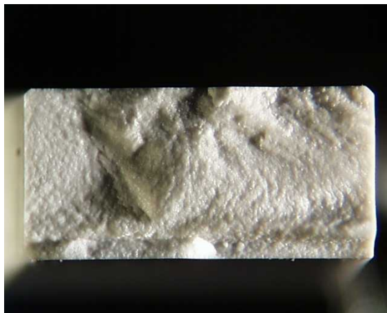
Figure 12.—A typical fracture surface of an as-machined Pyroceram flexure specimen tested in room temperature distilled water.
