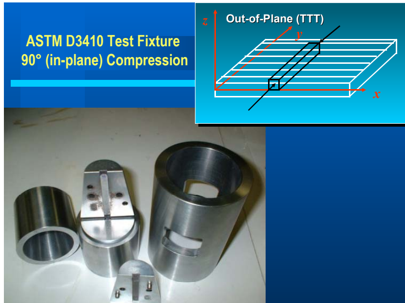
Fig.3 ASTM D3410 Test Fixture and 90° Specimen
