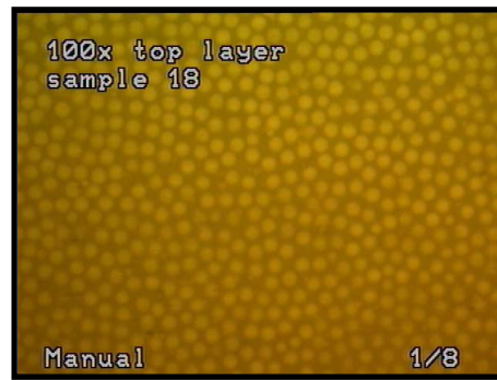
Figure 11 – Two Micron Diameter PMMA Spheres Dyed with Rhodamine (x-z slice). Taken with Yokagawa Confocal Unit—100x Objective
