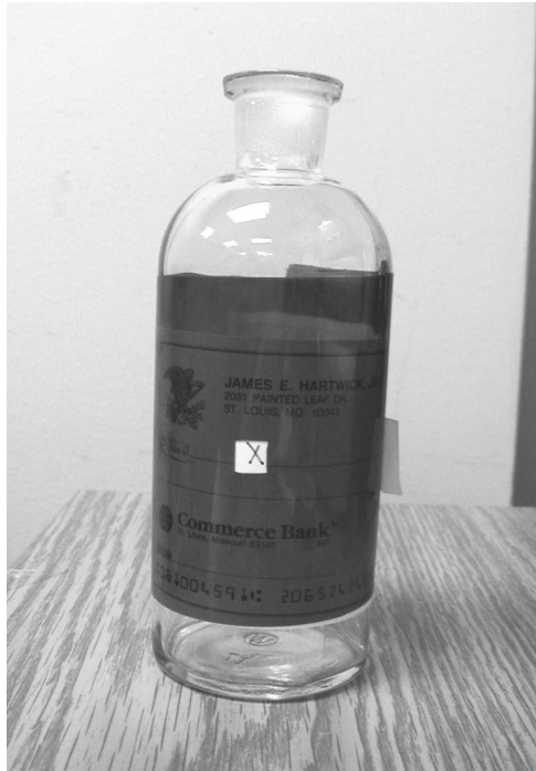
(a). Kapton protects the document from atomic oxygen exposure except for a small window cut in the questioned area.
