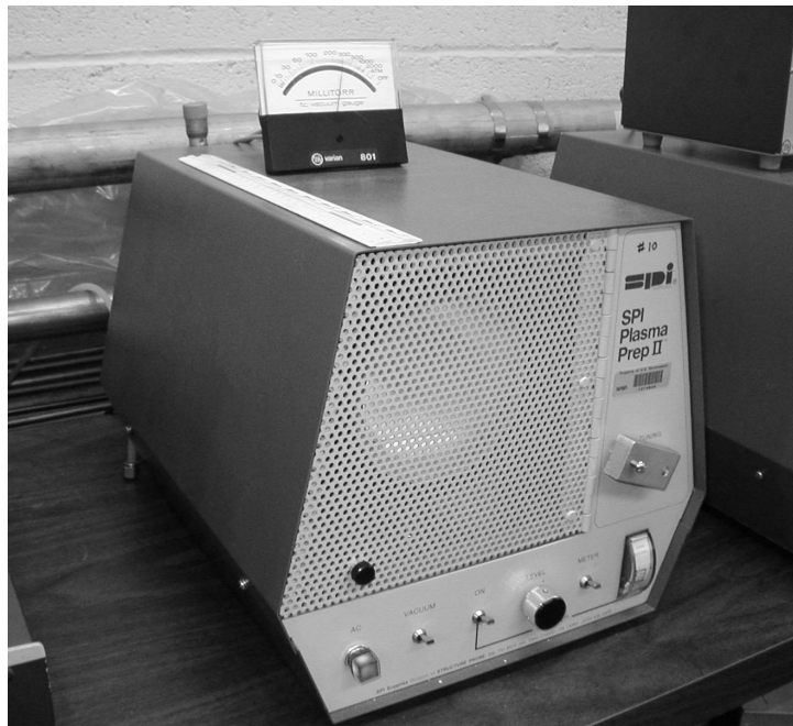
(b). Plasma asher during operation. Figure 2.—SPI Plasma Prep II Plasma Asher.
