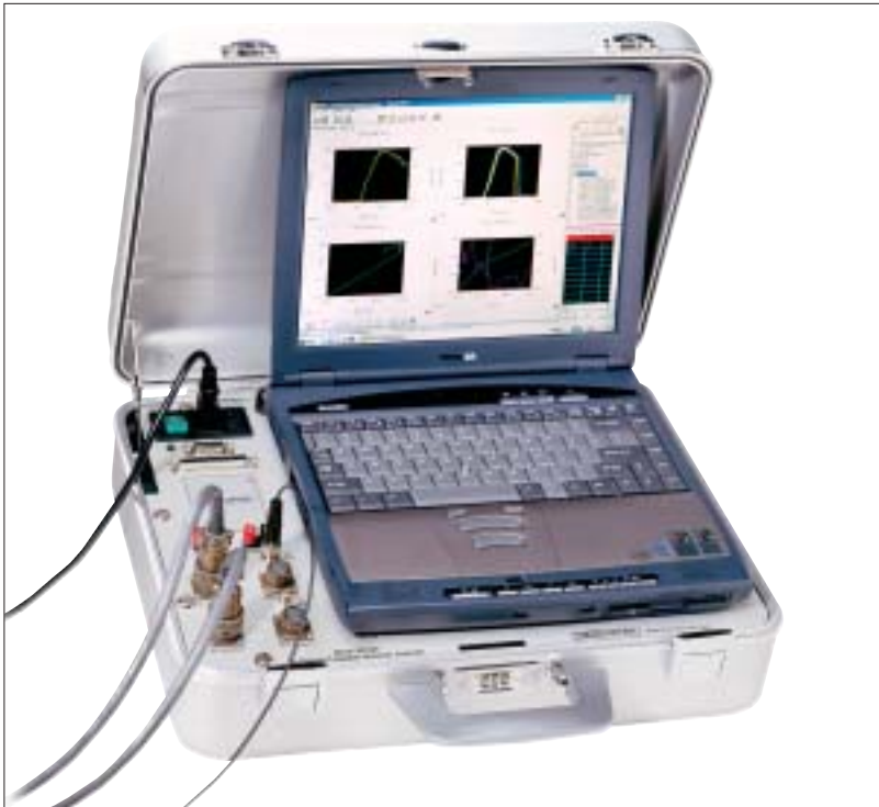
The MC900 Transient Recorder Analyzer is available in a portable laptop model (shown here encased in aluminum), or a desktop model made from high-impact plastic. Standard specifications include four strain gauge input channels, four high-level analog input channels, and four digital input and output channels, among other features.
