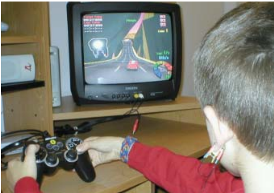
From flight simulation to brain stimulation: The S.M.A.R.T. BrainGames system uses electroencephalogram neurofeedback to make a video game respond to the activity of the player's body and brain.
