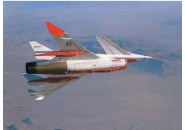
The Highly Maneuverable Aircraft Technology subscale research vehicle, seen here during a research flight, was flown by Dryden Flight Research Center from 1979 to 1983. The aircraft demonstrated advanced fighter technologies that have been used in the development of many modern high performance military aircraft.
