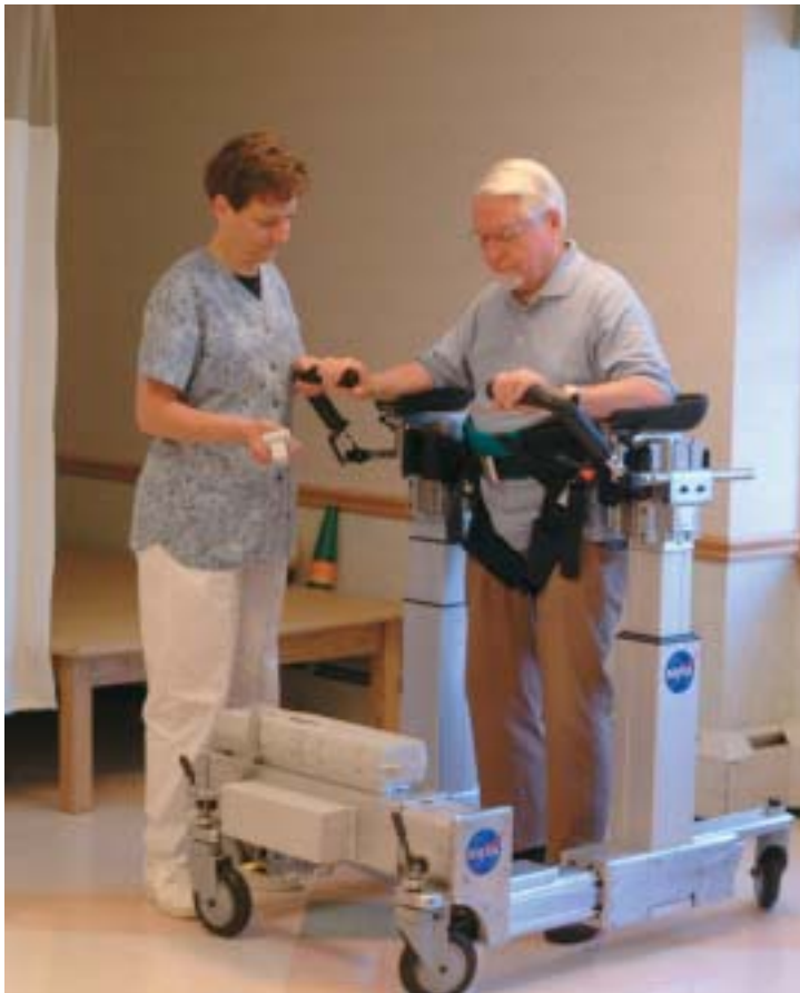
The Secure Ambulation Module creates a stable and secure environment for patients as they stand during ambulation therapy. The device increases staff efficiency, since a single therapist can bring a patient to a standing position.
