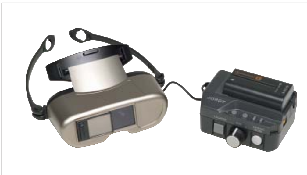
The JORDY™ headset, when worn like a pair of glasses, enables people with low vision to see objects at any range.
