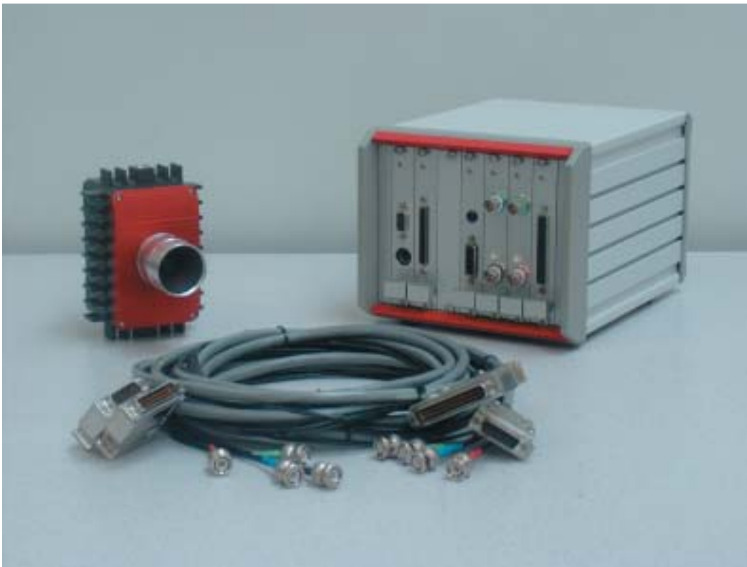
SciMeasure Analytical Systems, Inc.'s “Little Joe” wavefront sensor camera is finding increasing application in astronomy and medicine.
