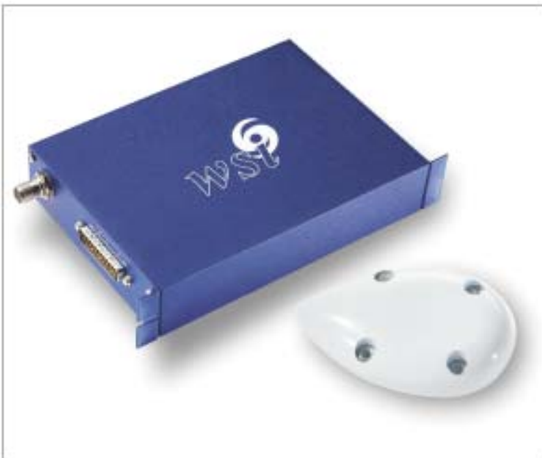
The WSI InFlight™ Cockpit Weather System enables pilots to receive and view high-resolution weather information right inside their aircraft cockpits.
