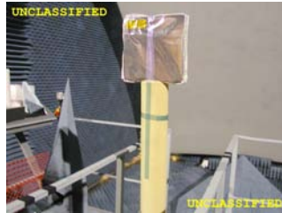
Figure 9 –Thermal Blanket on Low RCS Support at the AFRL Compact Range.
