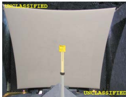
Figure 10 – ML-004 TPS Blanket in the AFRL ACR for UHF RCS Testing
