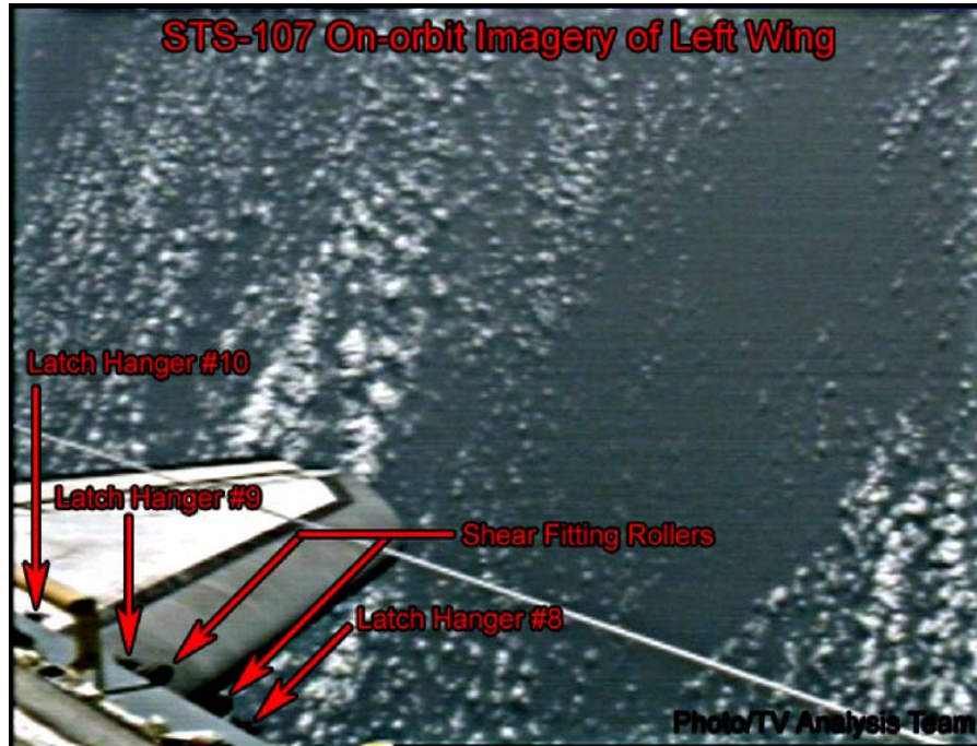
Figure 5.3.2.3b Payload bay door latches/rollers superimposed on Orbiter left wing
