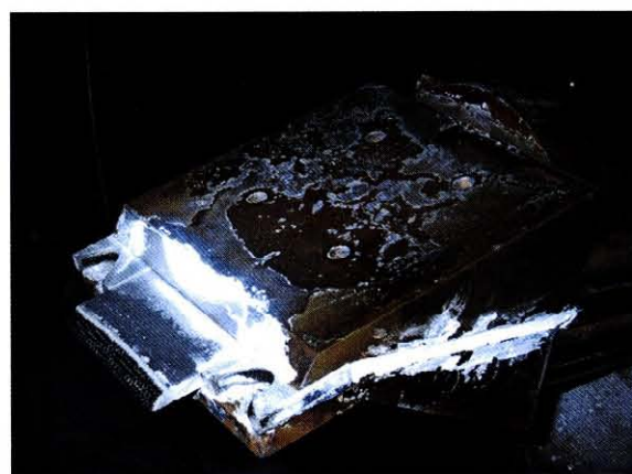
Figure 44 (b): Post-test Photograph Showing Knife-edges in Both RCC Test Article and Closeout.
