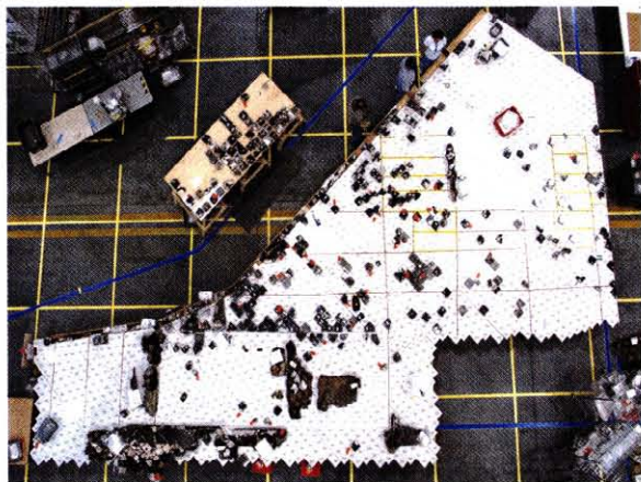
Figure 35: Overview of Tile Table. Left Wing, Lower Surface Tiles.
