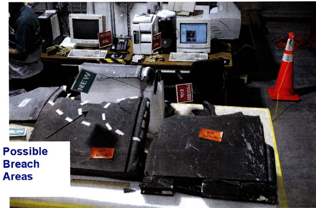
Figure 33: Probable Initial Breach in Panel 8.
