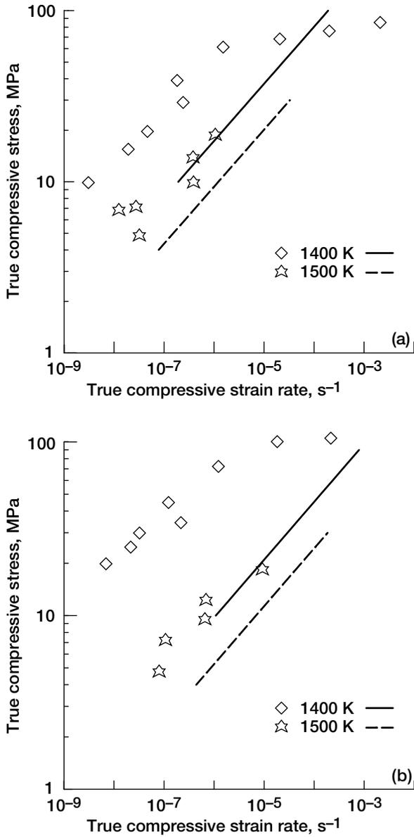
Figure 19.—Comparison of the elevated temperature compressive deformation behavior of (a)  $\langle 001 \rangle$ - and (b)  $\langle 111 \rangle$ -oriented NiAl-2Cr single crystals at 1400 and 1500 K (open symbols) to predicted Cottrell-Jaswon creep rates (curves).
