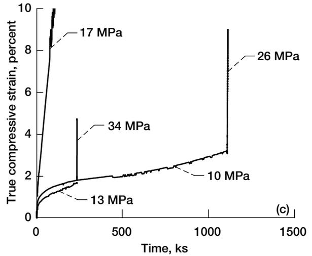
Figure 9.—Single and multiple constant load creep curves at 1400 K as a function of the engineering stress. (a)  $\langle 001 \rangle$  NiAl-2Cr. (b)  $\langle 111 \rangle$  NiAl-2Cr. (c)  $\langle 110 \rangle$  NiAl-6Cr.
