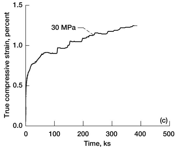
Figure 7.—Multiple constant load creep curves at 1200 K as a function of the engineering stress. (a)  $\langle 001 \rangle$  NiAl-2Cr. (b)  $\langle 111 \rangle$  NiAl-2Cr. (c)  $\langle 110 \rangle$  NiAl-6Cr.
