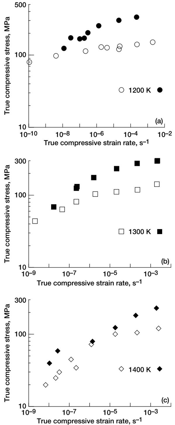
Figure 20.—Comparison of the elevated temperature compressive deformation behavior directionally solidified NiAl-33Cr-1Mo (open symbols, [12]) and  $\langle 111 \rangle$ -oriented NiAl-2Cr single crystals (open symbols). (a) 1200 K. (b) 1300 K. (c) 1400 K.
