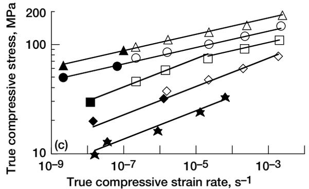
Figure 15.—True compressive flow stress-strain rate-temperature behavior. (a)  $\langle 001 \rangle$  oriented NiAl-2Cr. (b)  $\langle 111 \rangle$  oriented NiAl-2Cr. (c)  $\langle 011 \rangle$  oriented NiAl-6Cr.
