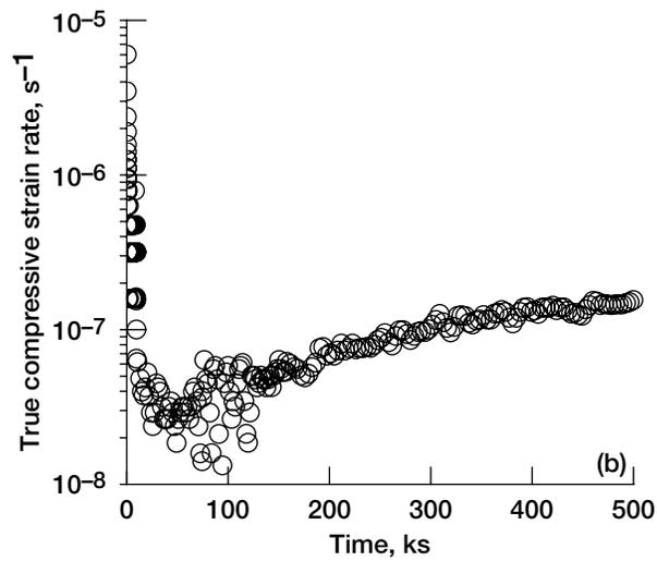
Figure 11.—Instantaneous true compressive strain rate-time curves for NiAl-2Cr creep tested at 1400 K as a function of the engineering stress. (a)  $\langle 001 \rangle$  oriented crystal under 20 MPa. (b)  $\langle 111 \rangle$  oriented crystal under 30 MPa.
