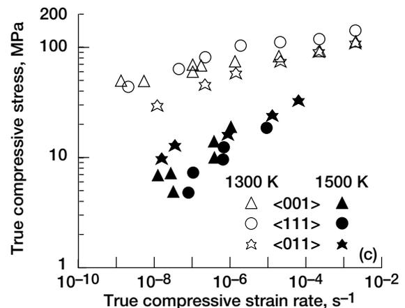
Figure 16.—Comparison of the true compressive flow stress-strain rate-temperature behavior for  $\langle 001 \rangle$  oriented NiAl-2Cr,  $\langle 111 \rangle$  oriented NiAl-2Cr, and  $\langle 011 \rangle$  oriented NiAl-6Cr. (a) 1100 and 1400 K. (b) 1200 K. (c) 1300 and 1500 K.
