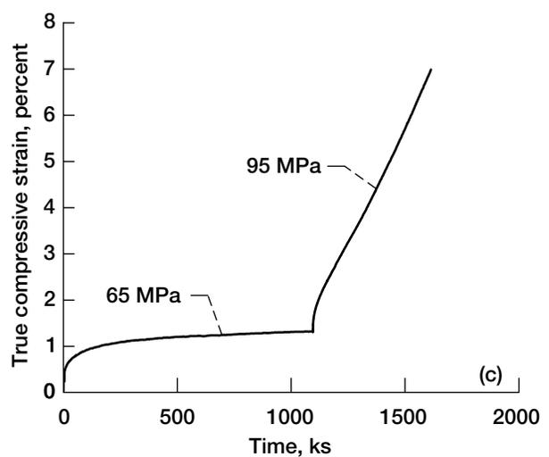
Figure 6.—Multiple constant load creep curves at 1100 K as a function of the engineering stress. (a)  $\langle 001 \rangle$  NiAl-2Cr. (b)  $\langle 111 \rangle$  NiAl-2Cr. (c)  $\langle 110 \rangle$  NiAl-6Cr.
