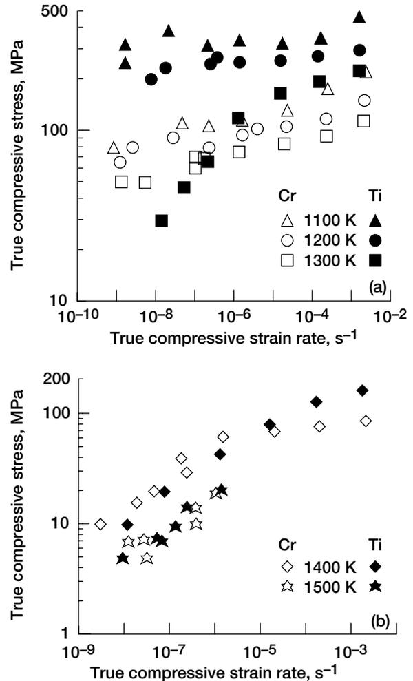
Figure 18.—Comparison of the elevated temperature compressive deformation behavior of  $\langle 001 \rangle$ -oriented NiAl-2Cr (open symbols) and NiAl-3.6Ti [27] (filled symbols) single crystals. (a) 1100 to 1300 K. (b) 1400 and 1500 K.
