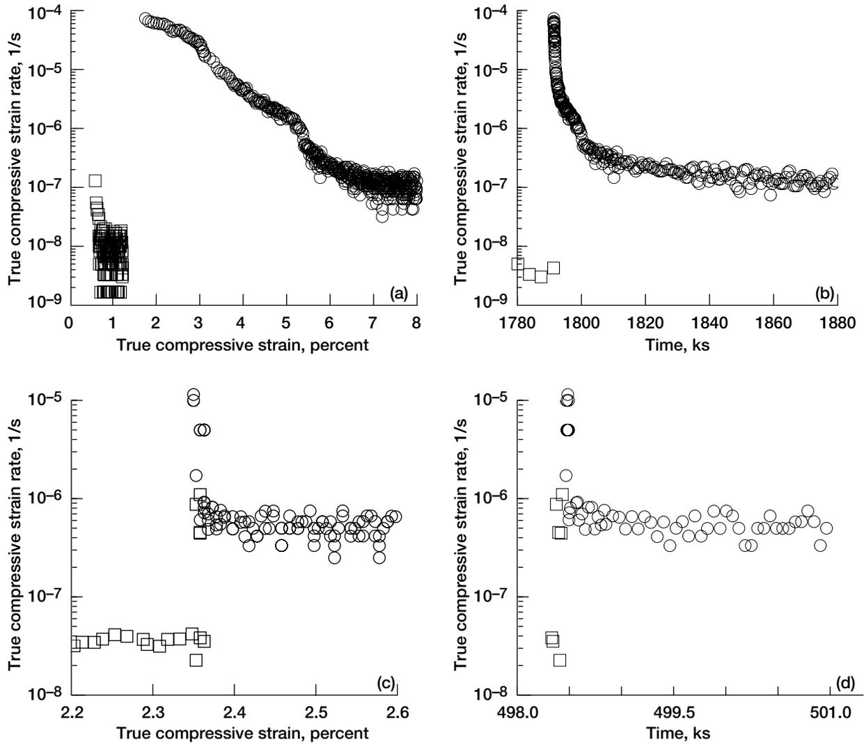
Figure 12.—Changes in the instantaneous strain rate as function of creep strain (a,c) and time (b,d) as a result of an increase in the engineering stress for <001> oriented NiAl-2Cr. (a,b) 50 to 75 MPa transition at 1300 K, and (c,d) 5 to 10.4 MPa transition at 1500 K. In all parts the open squares represent the data at the lower stress, while the open circles represent results after the load increase.
