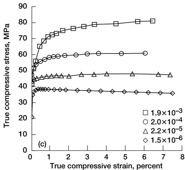
Figure 5.—The 1400 K stress–strain curves as a function of the nominally imposed strain rate. (a)  $\langle 001 \rangle$  NiAl-2Cr. (b)  $\langle 111 \rangle$  NiAl-2Cr. (c)  $\langle 110 \rangle$  NiAl-6Cr.
