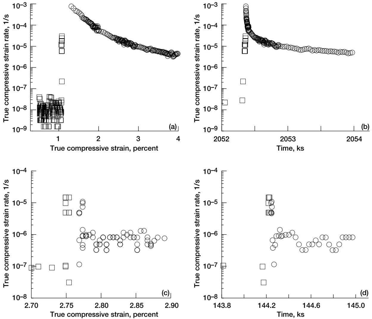
Figure 13.—Changes in the instantaneous strain rate as function of creep strain (a,c) and time (b,d) as a result of an increase in the engineering stress for <111> oriented NiAl-2Cr. (a,b) 98 to 134 MPa transition at 1200 K, and (c,d) 7.5 to 13 MPa transition at 1500 K. In all parts the open squares represent the data at the lower stress, while the open circles represent results after the load increase.
