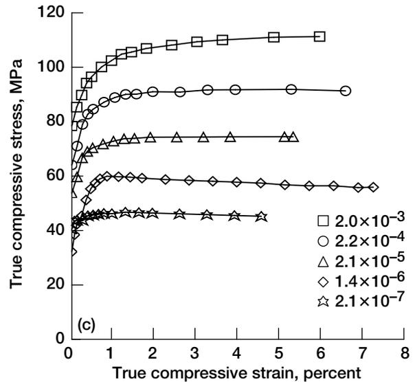
Figure 3.—The 1200 K stress–strain curves as a function of the nominally imposed strain rate. (a)  $\langle 001 \rangle$  NiAl-2Cr. (b)  $\langle 111 \rangle$  NiAl-2Cr. (c)  $\langle 110 \rangle$  NiAl-6Cr.
