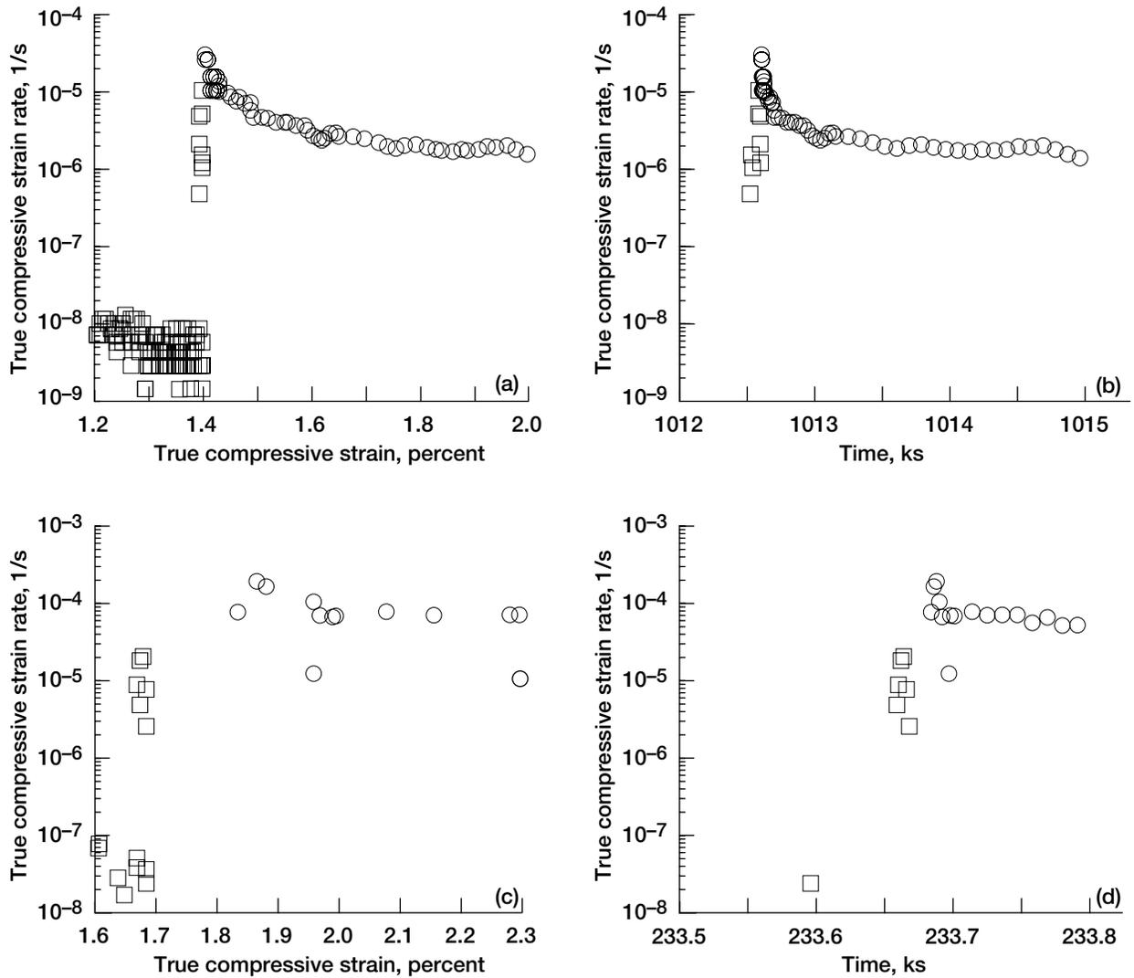
Figure 14.—Changes in the instantaneous strain rate as function of creep strain (a,c) and time (b,d) as a result of an increase in the engineering stress for <011> oriented NiAl-2Cr. (a,b) 20 to 33 MPa transition at 1400 K, and (c,d) 13 to 34 MPa transition at 1500 K. In all parts the open squares represent the data at the lower stress, while the open circles represent results after the load increase.
