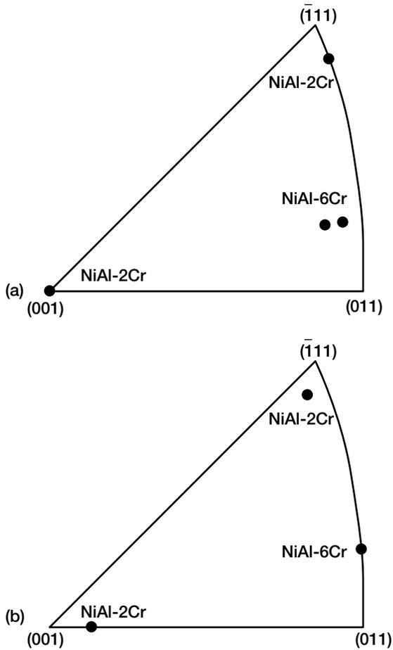
Figure 1.—Sterographic triangles illustrating the orientation of each set of compression samples, (a) as machined, (b) after being tested at 1300 K and a strain rate of  $\sim 1.5 \times 10^{-6} \text{ s}^{-1}$  to about 7% strain.
