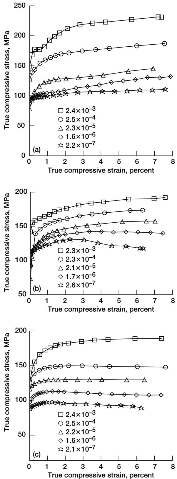
Figure 2.—The 1100 K stress–strain curves as a function of the nominally imposed strain rate. (a)  $\langle 001 \rangle$  NiAl-2Cr. (b)  $\langle 111 \rangle$  NiAl-2Cr. (c)  $\langle 110 \rangle$  NiAl-6Cr.
