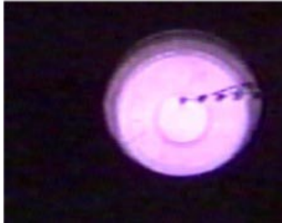
Figure 6c. “High Mode” operation. Notice absence of distinct ECR sites at the magnet rings.
