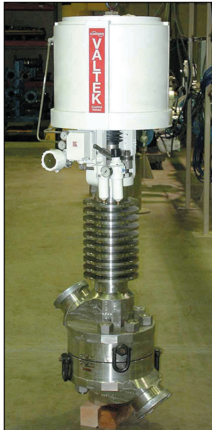
The Split-Body Design of this valve accommodates changes in trim. The heat-exchanger fins help keep the plug stem packing warm enough to function at cryogenic temperatures.
