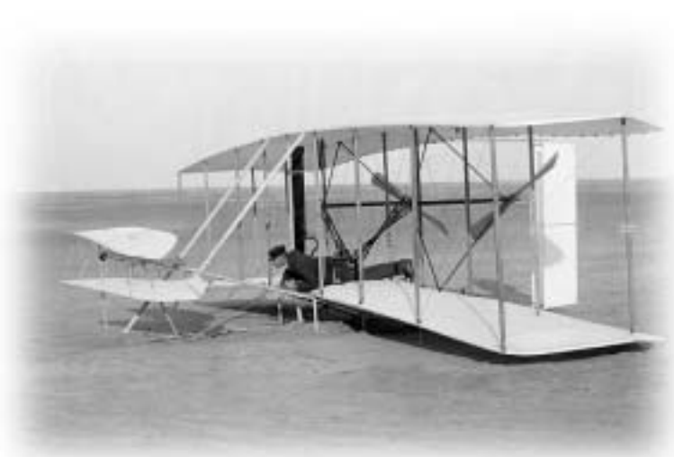
Wilbur in the damaged flyer after his unsuccessful trial on December 14, 1903. His hand still grips the wooden control lever.
