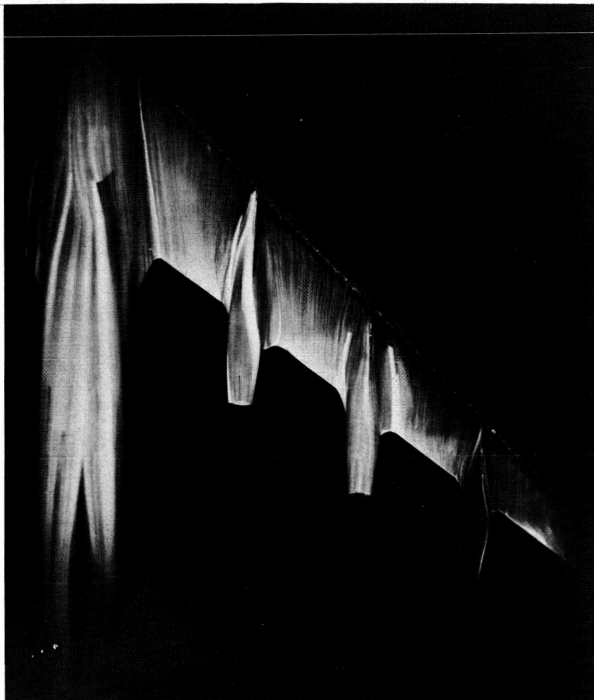
Figure 13.- Photograph of fluorescent-oil-film pattern on transonic-transport basic model with fences. \Lambda = 45^\circ ; \Gamma = 6^\circ ; M \approx 0.96 ; C_L \approx 0.3 .
