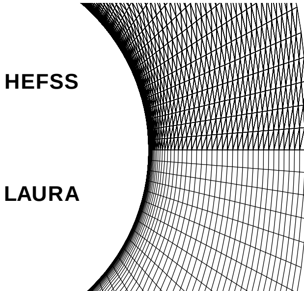
Fig. 6: Structured grid and equivalent uniformly biased unstructured grid in symmetry plane over cylinder for hypersonic test case.
